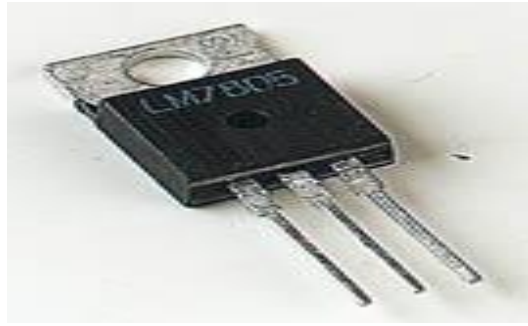
Figure 3.10:A Three Terminal Voltage Regulator
