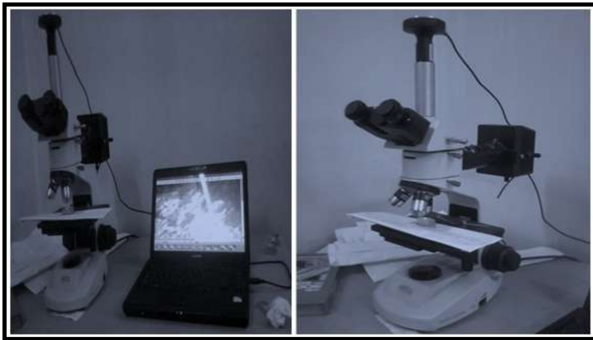
10Fig 3.2.3b Observation of the chip grain structure using a high power microscope with an embedded camera for snapping the chip structure.
