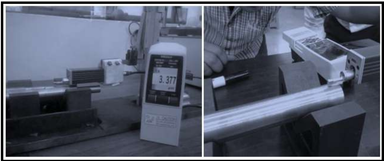
11 Fig 3.2.5a Apparatus for measuring the surface roughness
