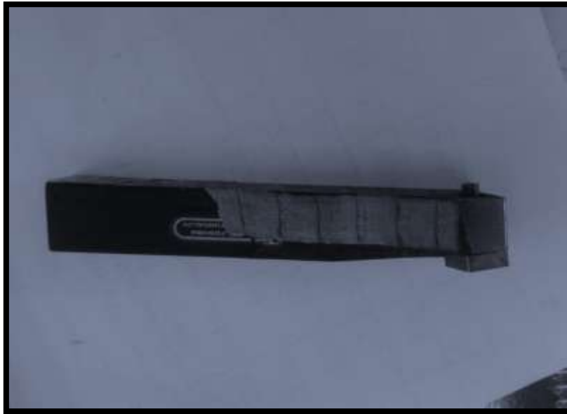
15Fig 3.2.8a The cutting tool showing the calibration scale of the overhang-length manually done in the machine workshop.
