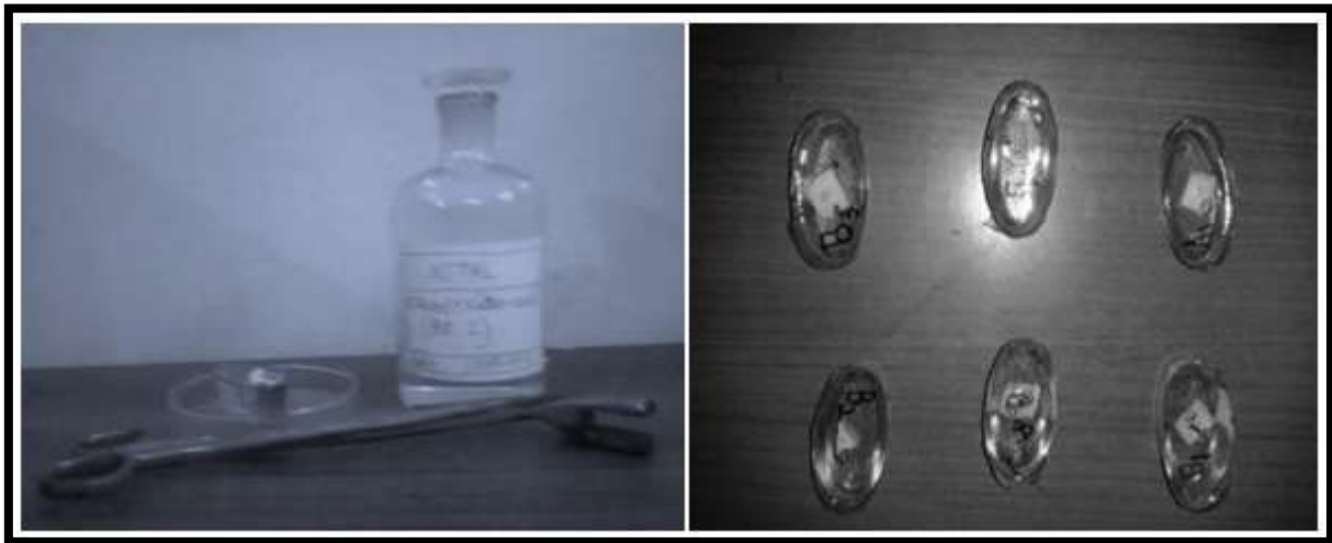
9Fig.3.2.3a chips grounded and ready to be observed. The bottle contains an alcohol called nitro used to wash the grounded chips in a small plastic basin as shown.
