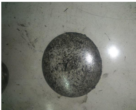
Figure V2.15: Step 6: Taking out the sample from furnace for grinding.
