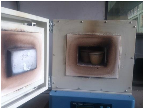
Figure V2.14: Step 5: Carbonize the sample at 450°C for 2 hours in the Muffle Furnace.
