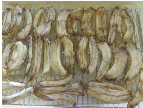
Figure V2.12: Step 3: drying the sample in the lab oven at 105°C for 24 hour
