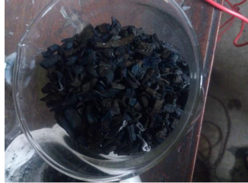
Figure V2.13: Step 4: Taking out the dried sample and cutting into small pieces.
