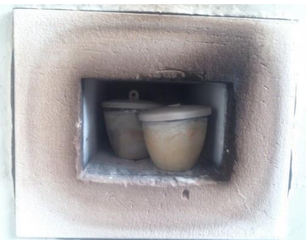
Figure V2.14: Step 5: Carbonize the sample at 450°C for 2 hours in the Muffle Furnace.
