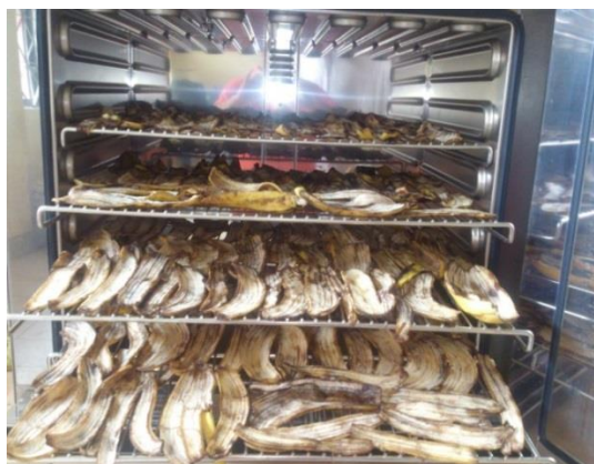
Figure V2.12: Step 3: drying the sample in the lab oven at 105°C for 24 hour
