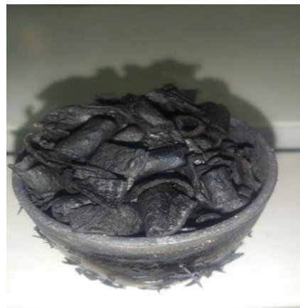
Figure V2.15: Step 6: Taking out the sample from furnace for grinding.
