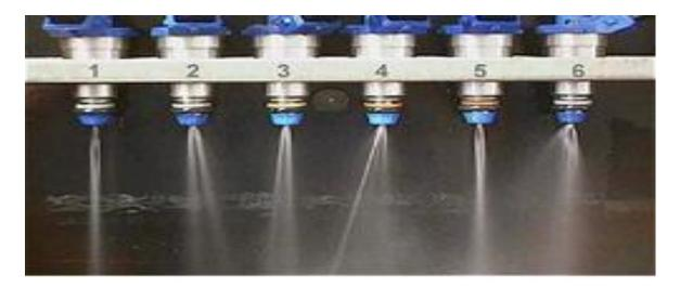
**Leaks:** leak can be through the Tapir internally or usually due to valve unable to fully close which in both cases cause the leak of fuel from the injector if there is no leak within the fuel injector then the problem may be in the fuel pump or distributer unable to set the timing
