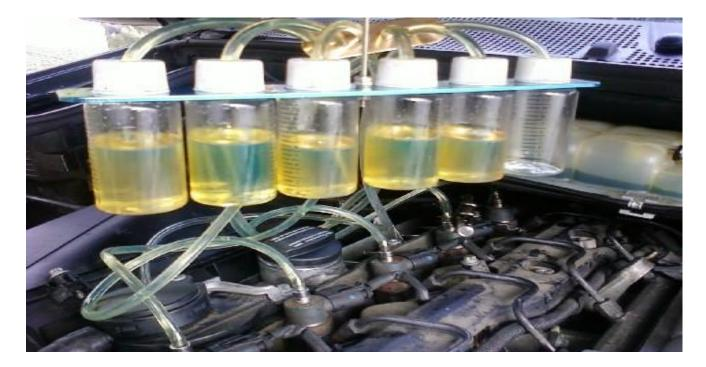
**Spray pattern**: If the flow rate is optimized and there is no leak the spray pattern will affect the combustion of the fuel usually spray pattern is result of change in the fuel injector nozzle projection that change the shape of the pattern of the spray which result in decrease in the fuel combustion efficiency
