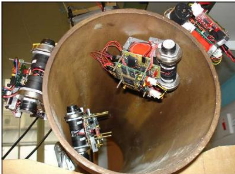
Fig.1.14: X-ray robots trying to find cracks on the surface of pipe
