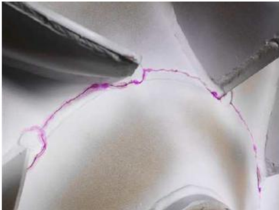
Fig.1.13 Dye Penetration in a stiffening cone of a turbine
