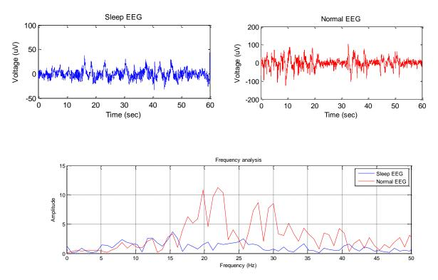
Figure 4.2: Frequency spectrum of sleepy & non-sleepy EEG signal
