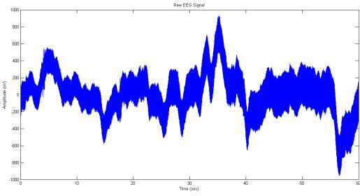
Figure 4.9: Raw EEG signal containing 50 Hz noise from AC line
