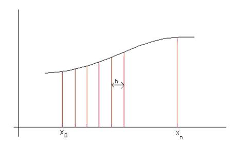
Figure 3.1: Splitting of area under a curve for trapezium rule
