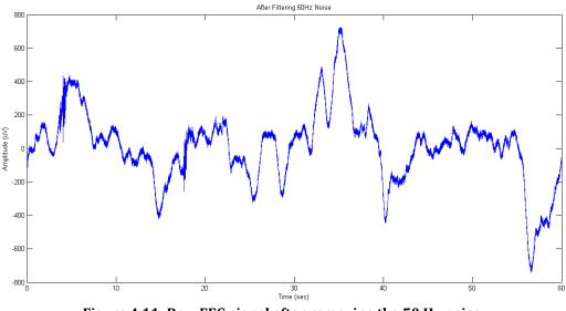
Figure 4.11: Raw EEG signal after removing the 50 Hz noise
