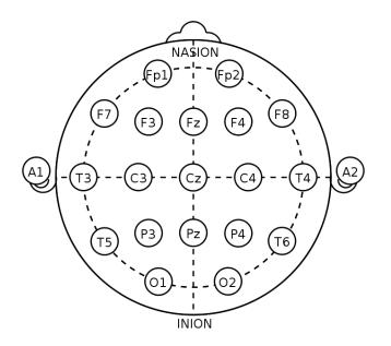
Figure 2.10: Electrode placement for 10-20 system
