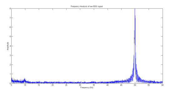
Figure 4.10: Frequency spectrum of the raw EEG signal containing 50 Hz noise
