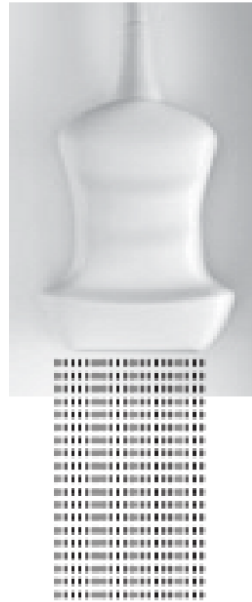
Figure 2.1 Ultrasound beams are coming out sequentially from the Ultrasound transducer
