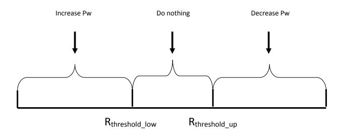
Figure 2.3:Adjusting transmission power level
