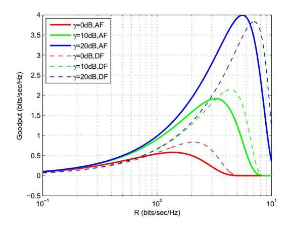
Figure 3.5:GoodputVs. Transmission Rate in AF and DF TWRN
