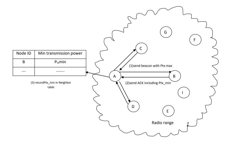
Figure 2.2: Operation of transmission power control
