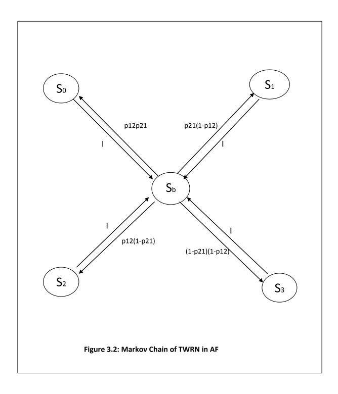
In Figure 3.3, it is explicitly seen at the beginning of each odd time slot that both  $T_1$  and  $T_2$  transmit to the relay such that at the beginning of each even time slot, the relay is always in the ready-for-broadcasting state S b and will consequently transition to  $S_0$ ,  $S_1$ ,  $S_2$ , or  $S_3$  with certain probabilities. We first determine the following four equations according to thestate transitions in the Markov chain to derive the probability of each state:
