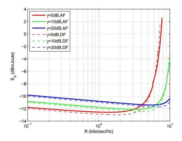
Figure 3.6: Average Bit Energy Vs. Transmission Rate
