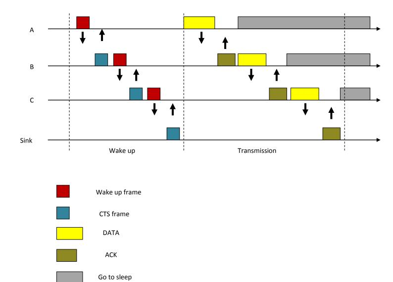
Figure 2.5: The duty-cycle scheduling scheme
