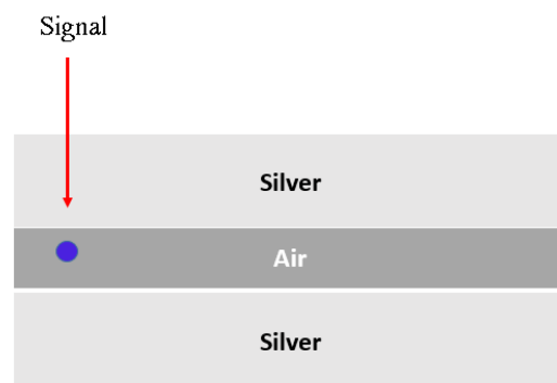
Figure 6.3: Metal Dielectric Metal Interface.
