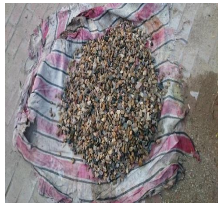
Fig 3.11: Coarse Aggregate after SSD Condition
