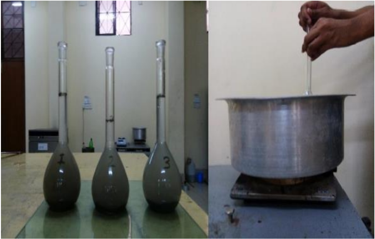
Figure 3.7 Laboratory test of determination of Specific gravity of soil.
