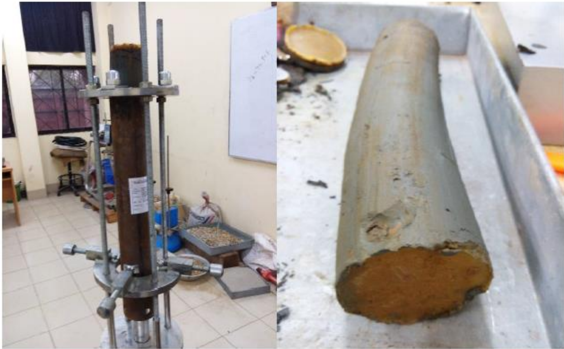
Figure 3.5 Sample extraction from Shelby tube
