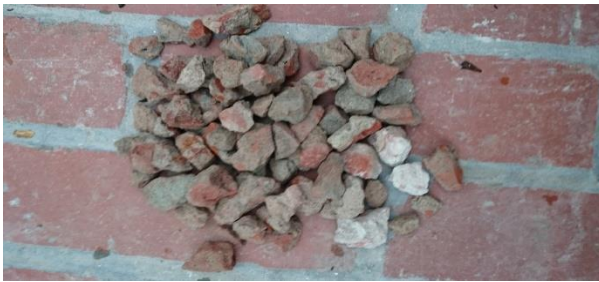
Photo 3.3: Recycled brick aggregate
