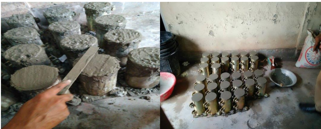
Photo 3.14: smoothing surface of cylinder
