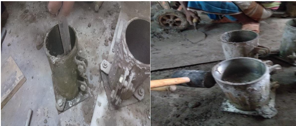
Photo 3.13: scaling and hammering
