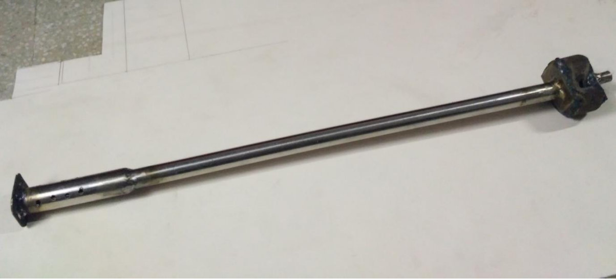
Figure 4.7 Vortex Tube (Experimental Setup)
