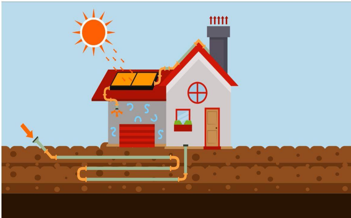
Figure 3: Experimental Setup of the Passive Cooling System
