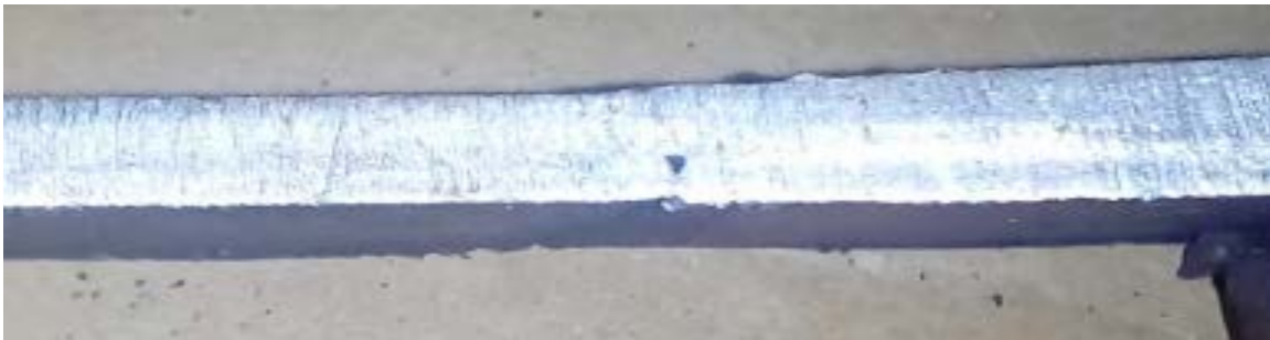
V_A = 25\mu\text{m} , V_F = 175\text{ Hz} , W_S = 2.0\text{mm/sec} , E_A = 30^0 (Sample No. 12)
