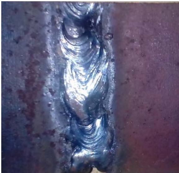
V_A = 15.0\mu\text{m} , V_F = 100\text{ Hz} , W_S = 2\text{ mm/sec} , E_A = 15^0 (Sample No. 1) (a)
