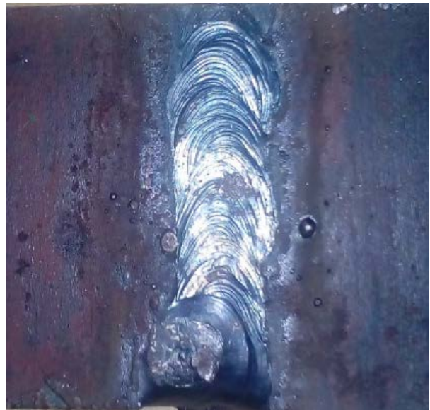
V_A = 20\mu\text{m} , V_F = 150\text{ Hz} , W_S = 3.5\text{mm/sec} , E_A = 11.9^\circ (Sample No.23) (b)
