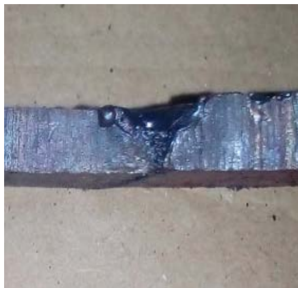
V_A = 0\mu\text{m} , V_F = 0 , W_S = 2.0\text{mm/sec} , E_A = 30^\circ (Sample No.39) (c)
