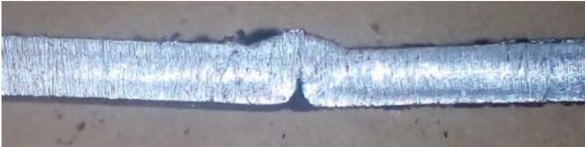
V_A = 15\mu\text{m} , V_F = 100\text{ Hz} , W_S = 2.0\text{mm/sec} , E_A = 30^0 (Sample No. 9)
