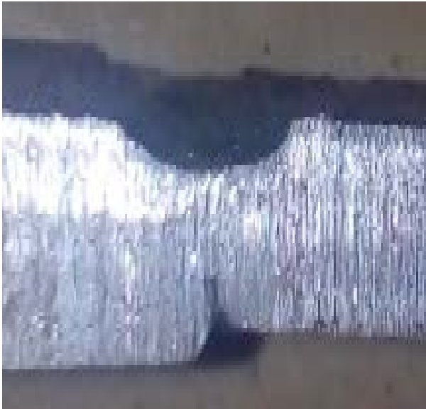
V_A = 15\mu\text{m} , V_F = 200\text{ Hz} , W_S = 5.0\text{mm/sec} , E_A = 30^\circ (Sample No.15) (a)
