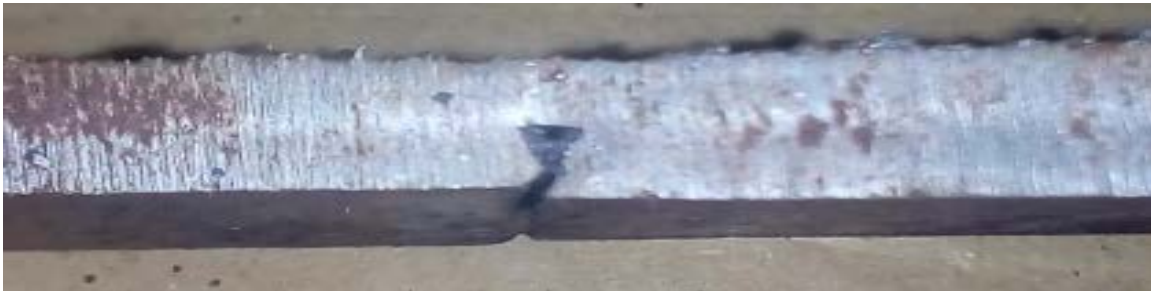
V_A = 25\mu\text{m} , V_F = 100\text{ Hz} , W_S = 5\text{mm/sec} , E_A = 30^0 (Sample No.14) (a)
