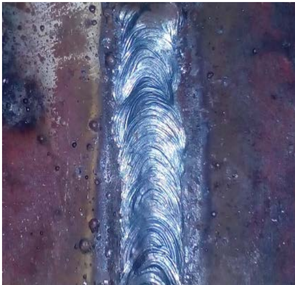
V_A = 20\mu\text{m} , V_F = 220.7\text{ Hz} , W_S = 3.5\text{mm/sec} , E_A = 22.5^\circ (Sample No.20)
