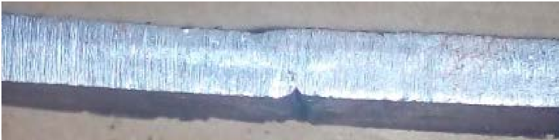
V_A = 25\mu\text{m} , V_F = 200\text{ Hz} , W_S = 2.0\text{mm/sec} , E_A = 15^0 (Sample No.4) (b)
