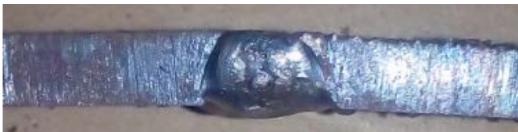
V_A = 20\mu\text{m} , V_F = 150\text{ Hz} , W_S = 1.4\text{mm/sec} , E_A = 22.5^\circ (Sample No.21)
