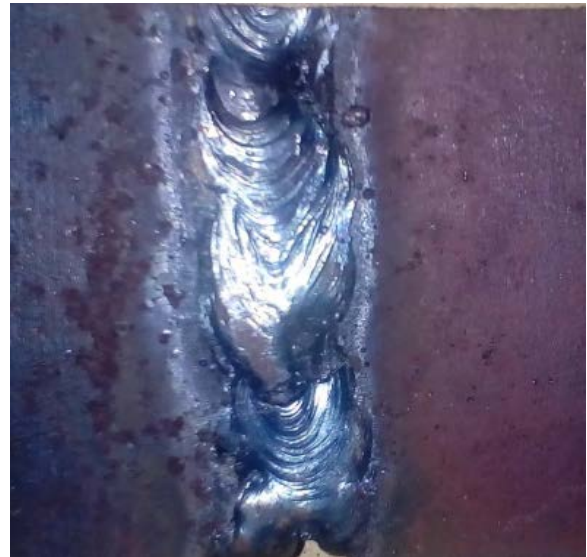
V_A = 15.0\mu\text{m} , V_F = 100\text{ Hz} , W_S = 2\text{ mm/sec} , E_A = 15^\circ (Sample No. 1)
