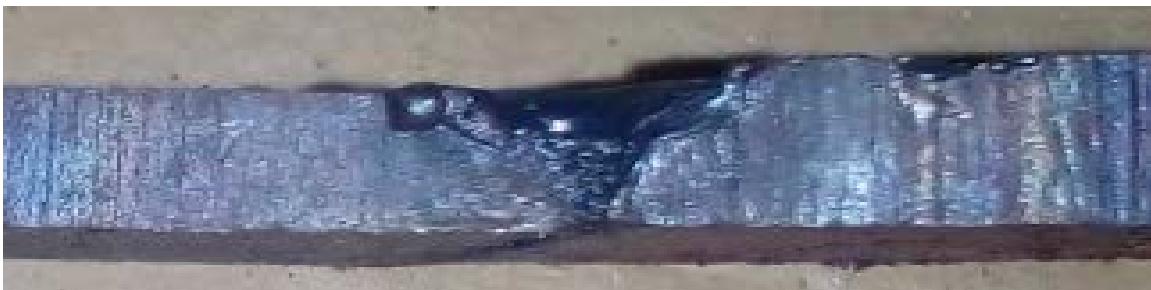
V_A = 0\mu\text{m} , V_F = 0 , W_S = 2.0\text{mm/sec} , E_A = 30^\circ (Sample No.39)
