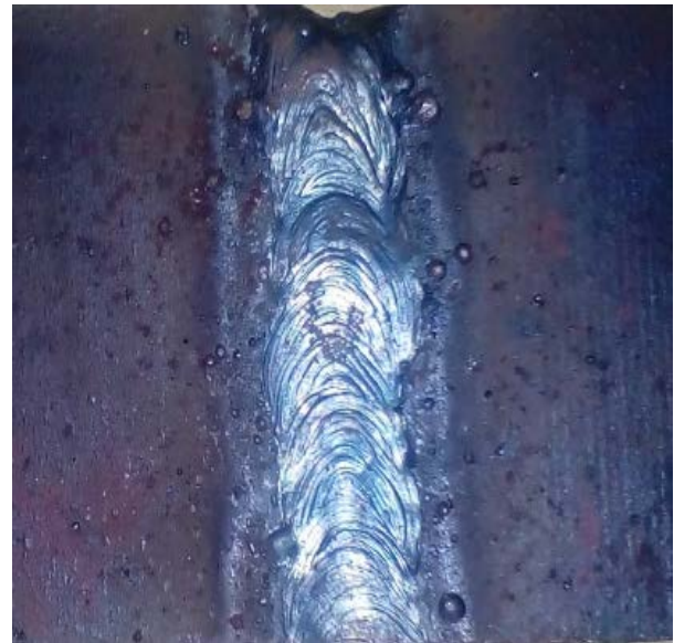
V_A = 25\mu\text{m} , V_F = 200\text{ Hz} , W_S = 5.0\text{mm/sec} , E_A = 30^\circ (Sample No.16)
