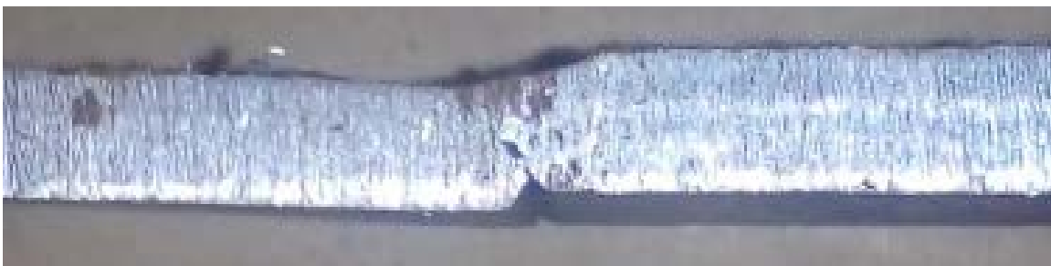
V_A = 0 , V_F = 0 , W_S = 5\text{mm/sec} , E_A = 15^0 (Sample No.34) (c)
