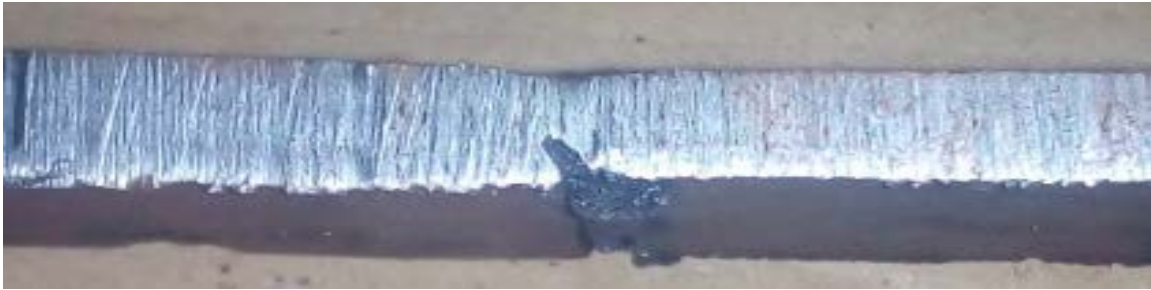
V_A = 15\mu\text{m} , V_F = 100\text{ Hz} , W_S = 2.0\text{mm/sec} , E_A = 15^0 (Sample No.1) (a)
