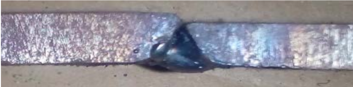
V_A = 15\mu\text{m} , V_F = 200\text{ Hz} , W_S = 5\text{ mm/sec} , E_A = 30^\circ (Sample No. 15)
