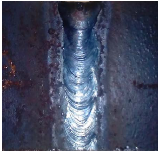
V_A = 15\mu\text{m} , V_F = 200\text{Hz} , W_S = 2.0\text{mm/sec} , E_A = 15^0 (Sample No.3) (b)
