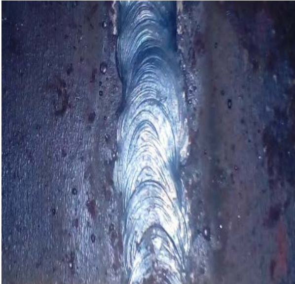
V_A = 15\mu\text{m} , V_F = 200\text{ Hz} , W_S = 2.0\text{mm/sec} , E_A = 15^\circ (Sample No.2) (a)
