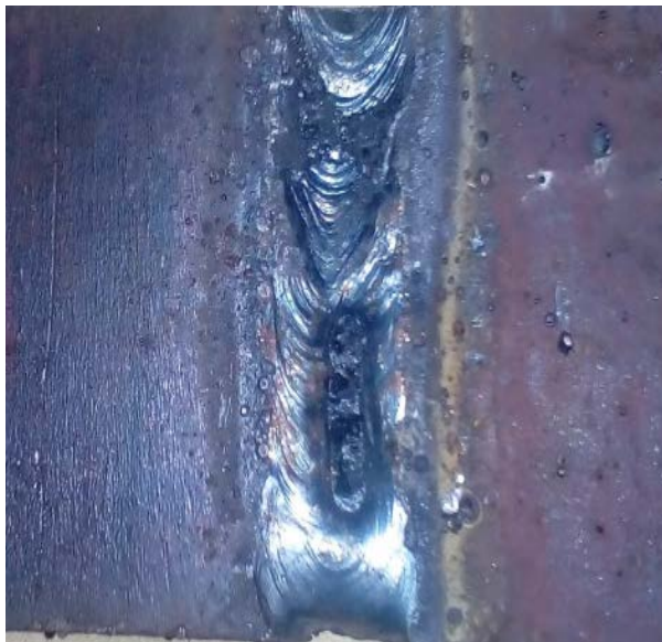
V_A = 15\mu\text{m} , V_F = 100\text{ Hz} , W_S = 5.0\text{mm/sec} , E_A = 15^\circ (Sample No.5)
