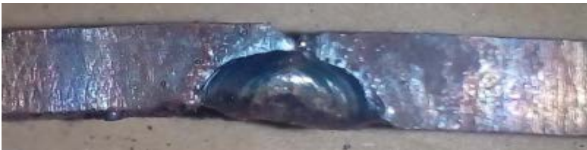
V_A = 20\mu\text{m} , V_F = 150\text{ Hz} , W_S = 3.5\text{mm/sec} , E_A = 11.9^\circ (Sample No.23)
