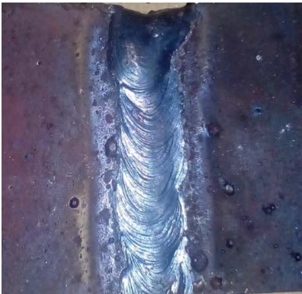
V_A = 25\mu\text{m} , V_F = 200\text{ Hz} , W_S = 5.0\text{mm/sec} , E_A = 15^0 (Sample No.8) (a)
