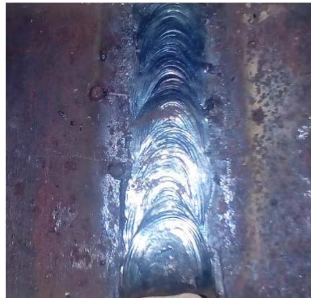
V_A = 25\mu\text{m} , V_F = 100\text{ Hz} , W_S = 2.0\text{mm/sec} , E_A = 15^0 (Sample No.2) (b)
