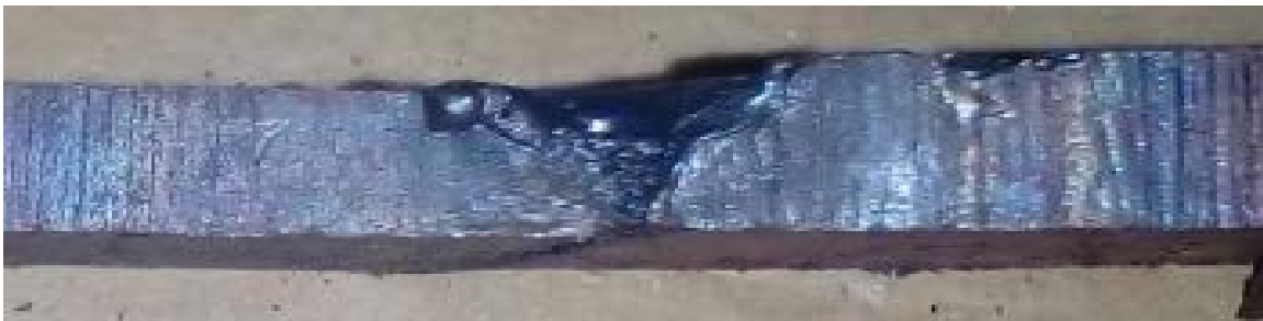
V_A = 15\mu\text{m} , V_F = 100\text{ Hz} , W_S = 2.0\text{mm/sec} , E_A = 15^0 (Sample No.1)
