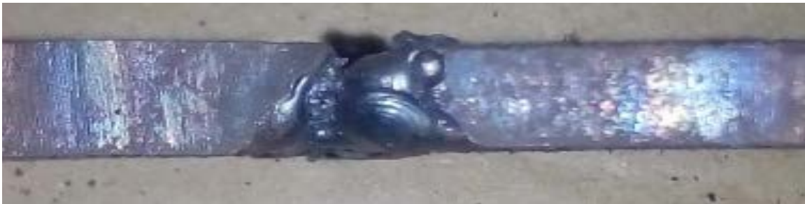
V_A = 20\mu\text{m} , V_F = 150\text{ Hz} , W_S = 3.5\text{mm/sec} , E_A = 33.1^\circ (Sample No.24)
