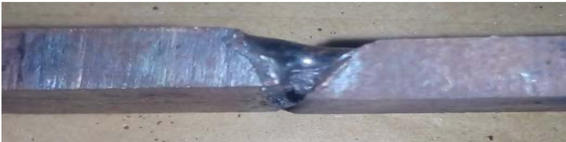
V_A = 0 , V_F = 0 , W_S = 5.6\text{mm/sec} , E_A = 15^\circ (Sample No.35) (c)
