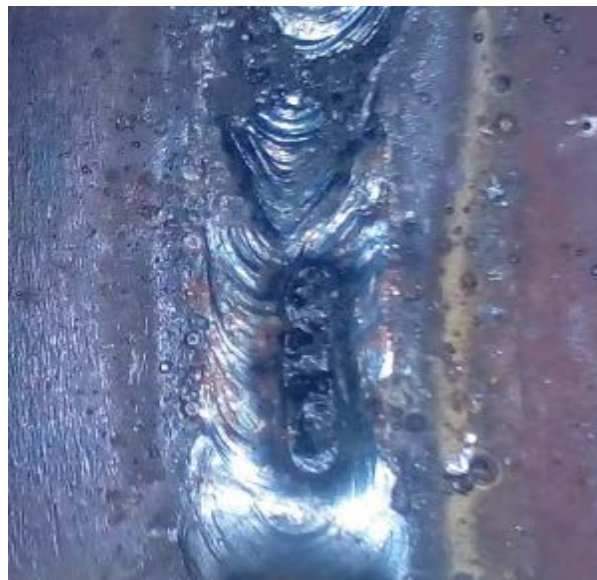
V_A = 0 , V_F = 0 , W_S = 2.0\text{mm/sec} , E_A = 33.1^\circ (Sample No.40) (c)
