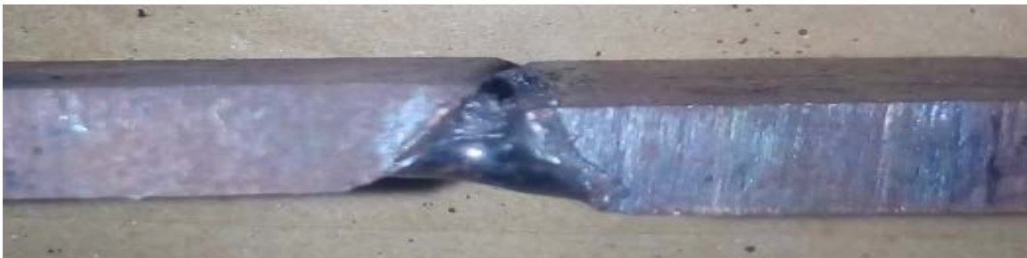
V_A = 0 , V_F = 0 , W_S = 5.6\text{ mm/sec} , E_A = 15^\circ (Sample No. 35)
