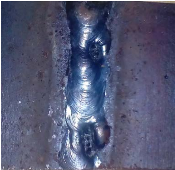
V_A = 20\mu\text{m} , V_F = 150\text{ Hz} , W_S = 3.5\text{mm/sec} , E_A = 33.1^\circ (Sample No.24) (a)
