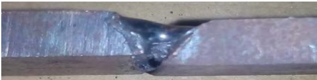
V_A = 15\mu\text{m} , V_F = 100\text{ Hz} , W_S = 5.0\text{mm/sec} , E_A = 30^\circ (Sample No.13)
