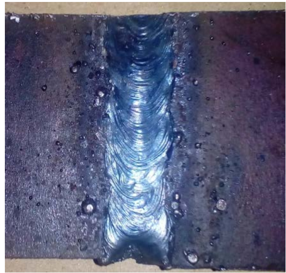
V_A = 25\mu\text{m} , V_F = 200\text{ Hz} , W_S = 2.0\text{mm/sec} , E_A = 15^0 (Sample No. 4) (b)
