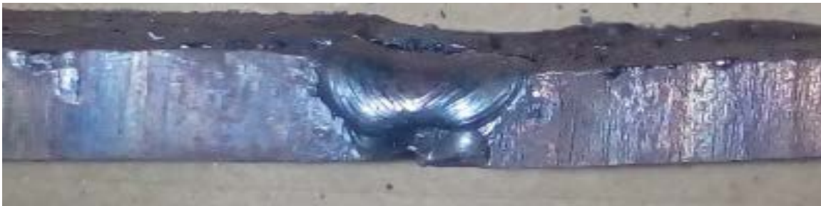
V_A = 25\mu\text{m} , V_F = 200\text{ Hz} , W_S = 2.0\text{mm/sec} , E_A = 30^0 (Sample No.12)
