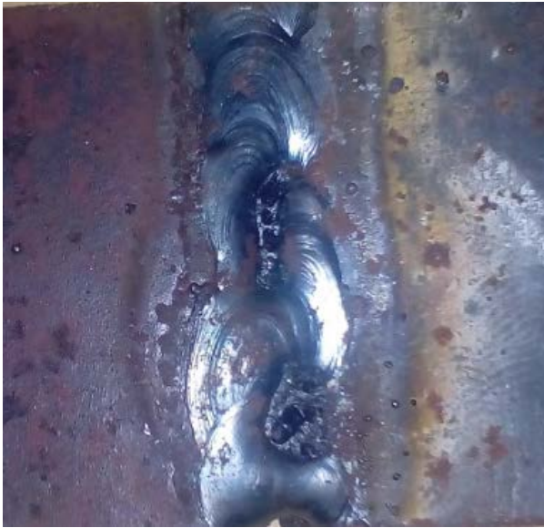
V_A = 15\mu\text{m} , V_F = 100\text{ Hz} , W_S = 5\text{mm/sec} , E_A = 30^0 (Sample No.13) (a)
