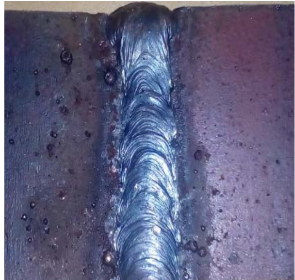
V_A = 15\mu\text{m} , V_F = 200\text{ Hz} , W_S = 5.0\text{mm/sec} , E_A = 15^\circ (Sample No.7) (b)
