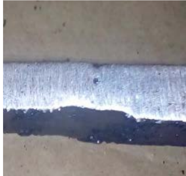
V_A = 20\mu\text{m} , V_F = 150\text{ Hz} , W_S = 5.6\text{mm/sec} , E_A = 22.5^\circ (Sample No.22) (b)
