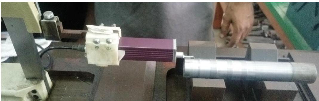
Figure 23 Surface Roughness measurement by Profilometer
