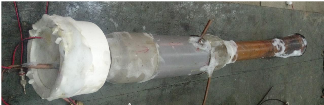
Figure 20 Bubble Testing for Leak Detention
