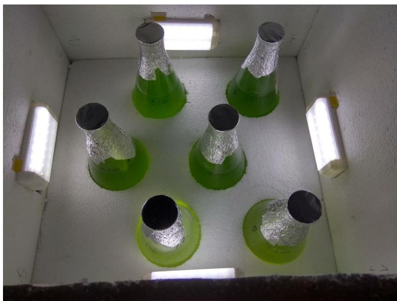
Figure 4: Customized Photo-bioreactor for optimum light supply during shaking.
