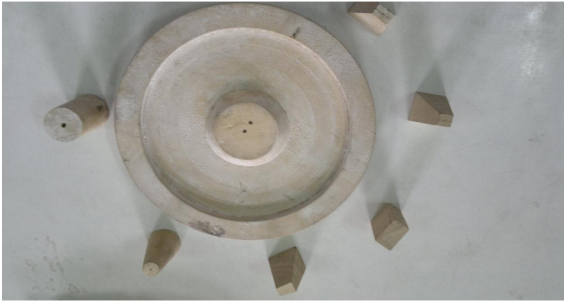
Fig 2.3 Wooden Pattern and Various sprues
