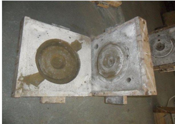
Fig: 3.2 Mold where using Sodium silicate mixing sand
