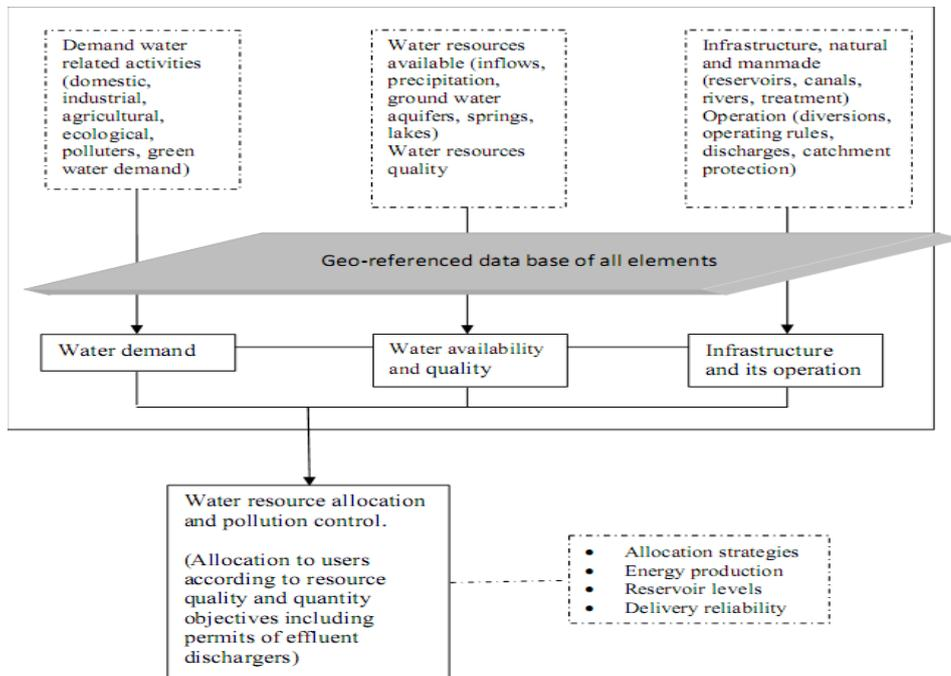
Figure 2.1 Schematic elements of water management (Source: Mugatsia, 2010)
