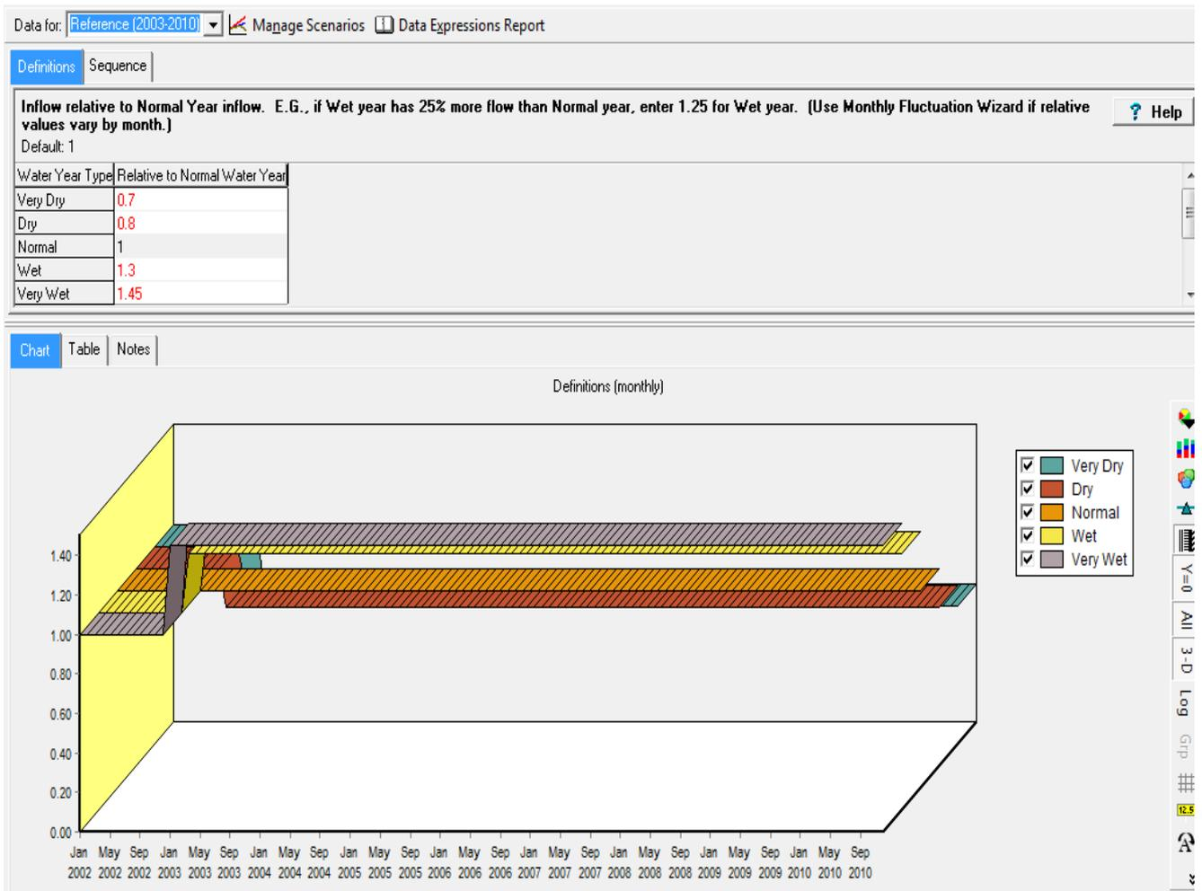
Figure 5.19 The input data for the water year method
