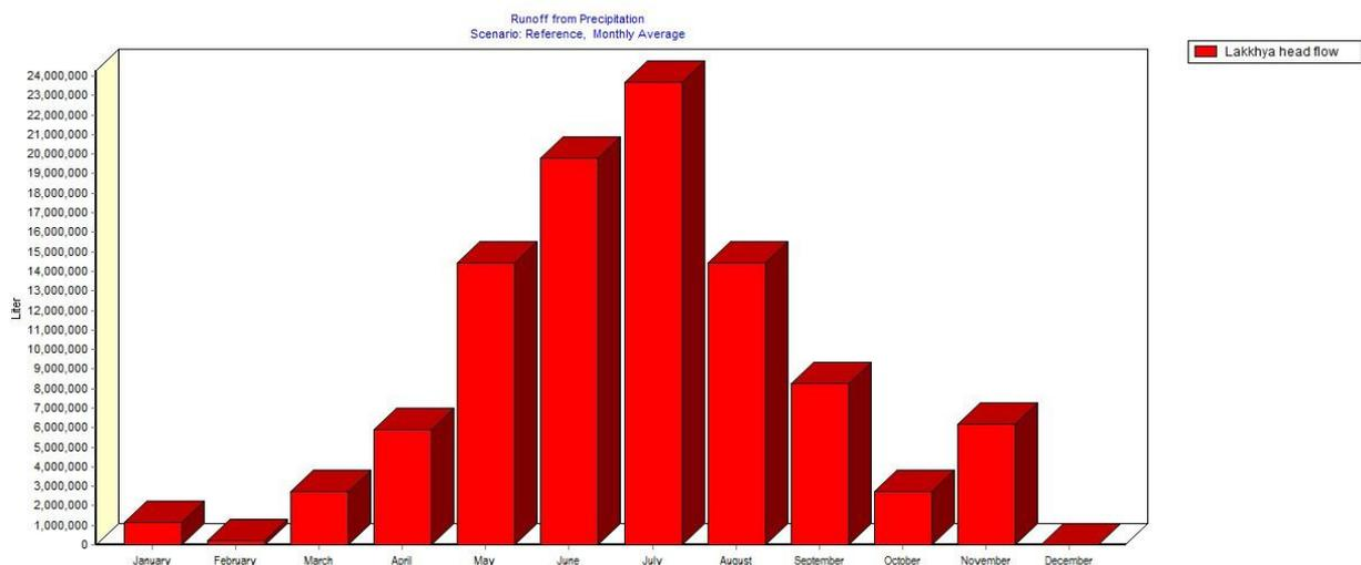
Figure 5.3 Runoff from climate data for year 2002 of Lakkhya headflow generated from catchment modelling
