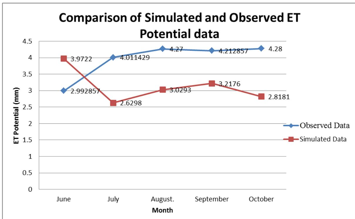
Figure 5.7 Comparison of Observed and WEAP simulated ET Potential data
