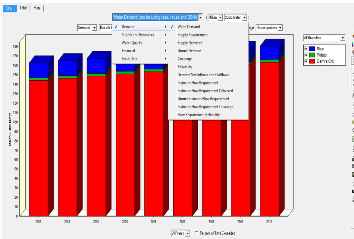
Figure 5.13 Simulated result of water demand for three demand sites and various other options to be calculated by running the model.
