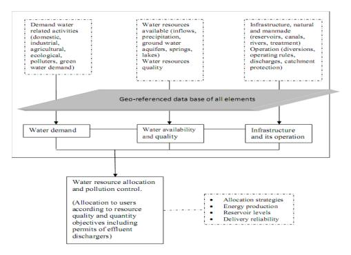
Figure 2.1 Schematic elements of water management (Source: Mugatsia, 2010)
