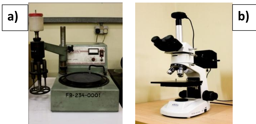
Figure: 3.16 Instruments used for chip analysis. a) Polishing wheel, b) optical microscope
