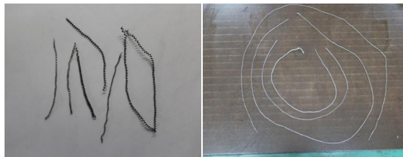
Fig. 4.23 (a) Discontinuous chips during non magnetic cutting
