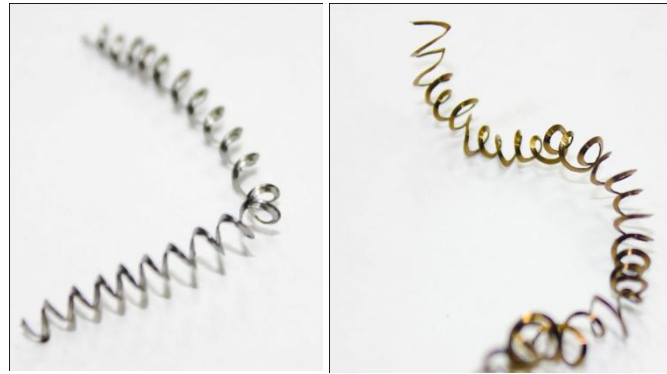
Fig. 4.25: (a) chips produced during non magnetic cutting condition (b) chips produced during magnetic cutting condition
