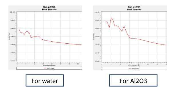
1. After simulating in the CFX-PRE we can obtain graphs of heat transfer. Comparing the above two cases we can see that the heat transfer rate is significantly increased in the latter case.
