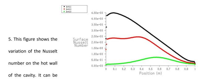
seen that by increasing partition height, Nusselt number along the hot wall decreases. It is because; the partition limits the fluid flow in the cavity.
