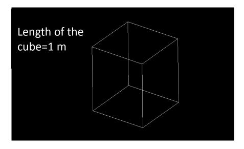
The simulation domain and the expected temperature distribution are shown schematically in Figure 1. The two vertical walls of the Cube enclosure are kept at different constant temperatures (TH – TC),
