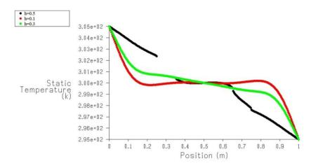
4. The above figure indicates the mid plane temperature variation with partition height. As it was concluded before, the increasing partition height leads to a decrease in the temperature gradient. At h=0.1, gradient increase is not very clear but the highest amount of the decrease is seen at h=0.5. It should be noted that the gap which occurs at h=0.5, is because of the partition's adiabatic surface.
