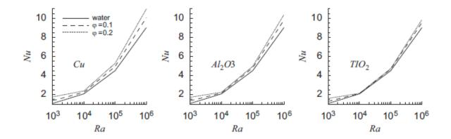
6. This shows the relationship between solid particle volume fraction and heat transfer. We observe for all three nanofluids that increasing solid particle volume fraction from 0.1 to 0.2 increases heat transfer. About the same increase is obtained if we compare pure water and nanofluid. The increase in heat transfer is highest when using Cu nanofluid and lowest when using TiO2 nanofluid.
