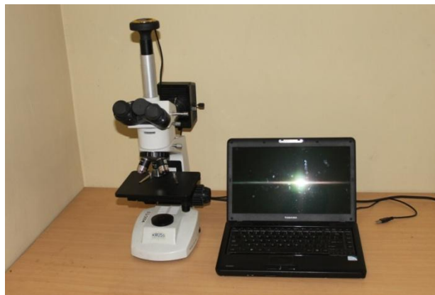
Fig 3.11: Optical microscope connected with laptop for taking image.
