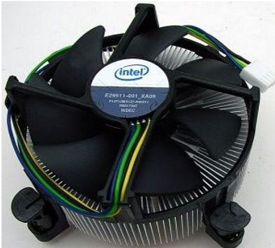
Fig 2.12: Traditional heat sink and fan
