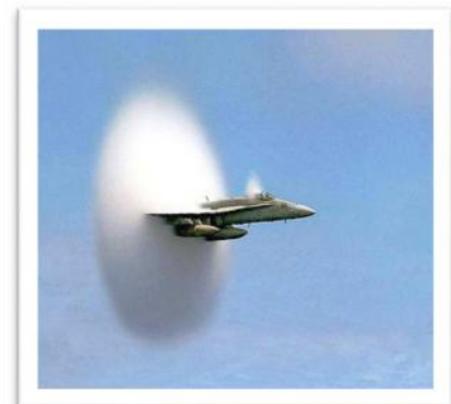
Figure 2.4: F-18 fighter is flying with transonic speed leaving visible signs of shock waves
