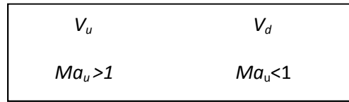
Figure 3.4: Stationary normal Shock wave in a pipe
