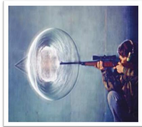
Figure 2.3: Schlieren image of a .30-06 caliber rifle discharge
