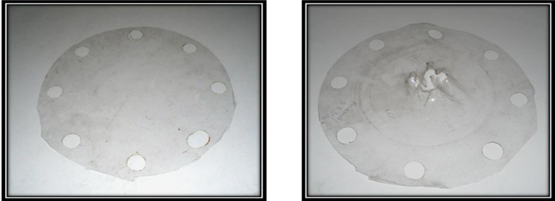
Figure 7.18: Condition of Celluloid Sheet Diaphragm before and after Shock Wave generation
