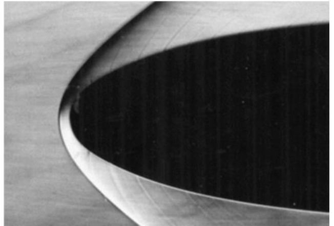
Figure 1.1: Schlieren photograph of supersonic flow over blunt object. Shock wave is detached from object
