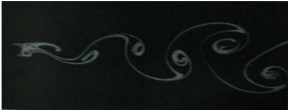
Figure 3.2: Flow over a cylinder, Re= 140 illustrating the Karman vortex street
