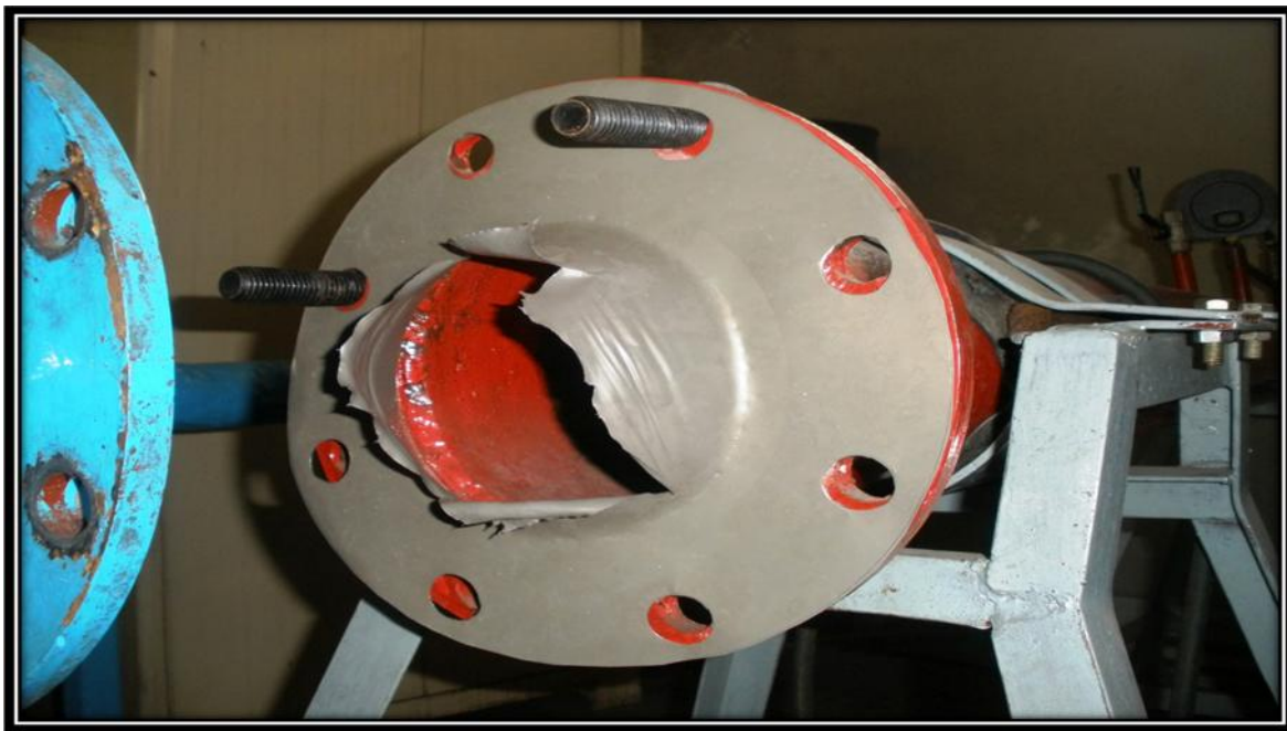
Figure 7.13: Diaphragm condition after Shock generation
