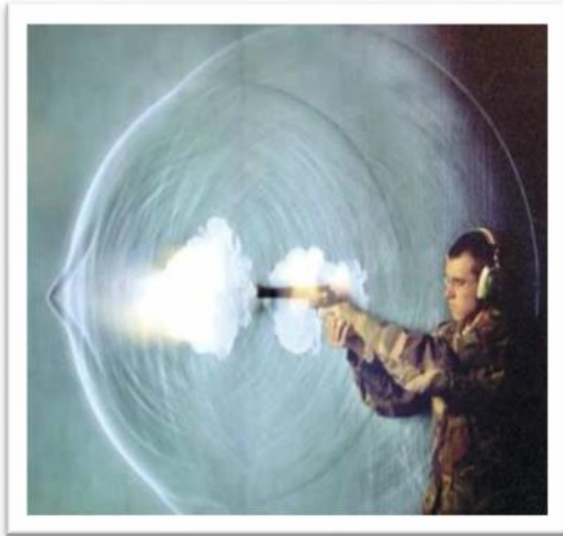
Figure 2.2: Full-scale schlieren image shows the discharge of a .44 Magnum revolver
