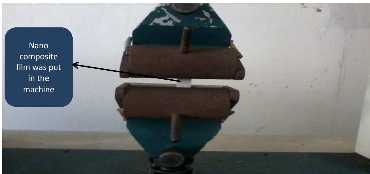
Figure 4.23: Nano composite film were kept in the universal testing machine
