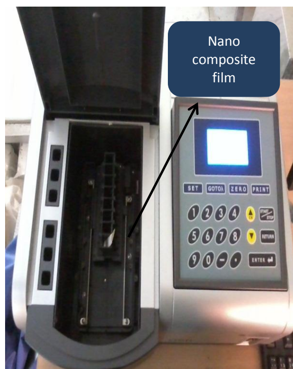
Figure 4.26: Sample were put in the UV -Visible Spectrophotometer
