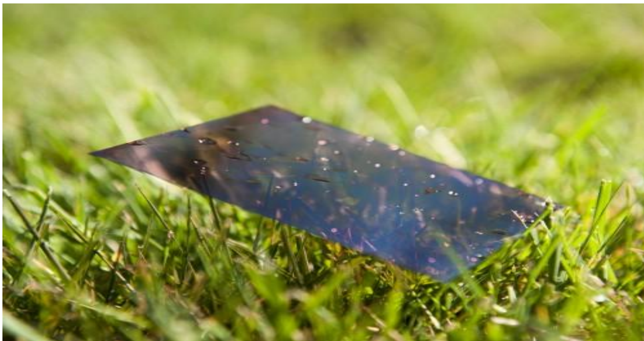
Figure 3.5: Flexible organic solar cell
