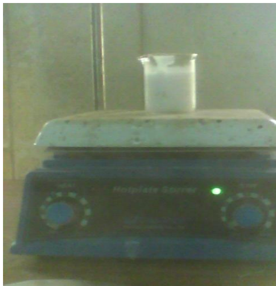
Figure 4.6: TiO 2 mixed solution was stirred magnetically
