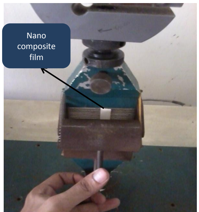
Figure 4.22: Sample was being put in the machine
