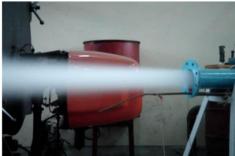
Figure 5.2: Photograph of Post-shocked high speed air delivered from end section of the shock tube.
