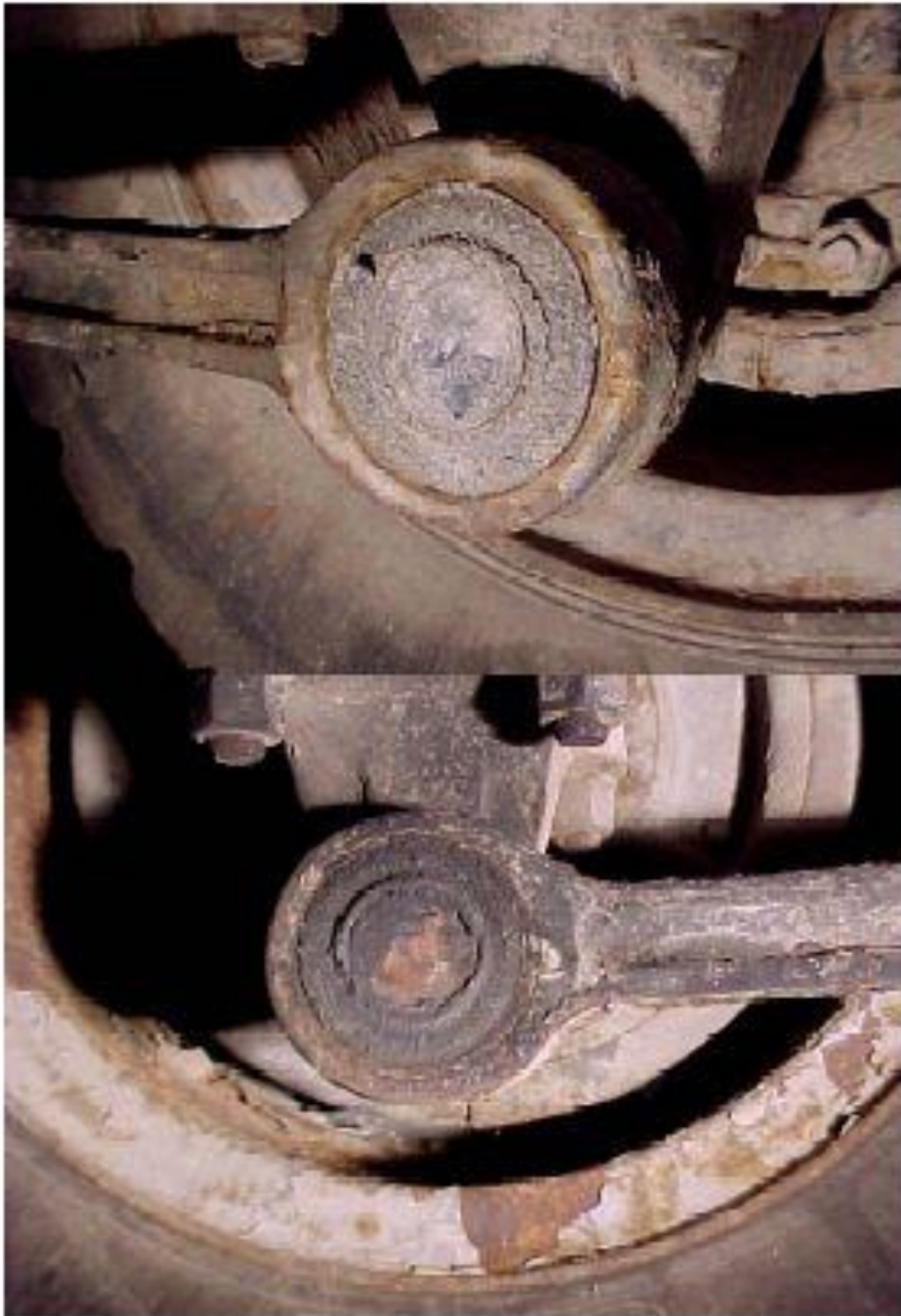
Figure 8. The above photos show rod ends that are starting to show some signs of deterioration. However, they would still be considered to be in usable condition. Notice the rubber peeling off the end of the inner ball joint. This is not an indication of a major problem.
