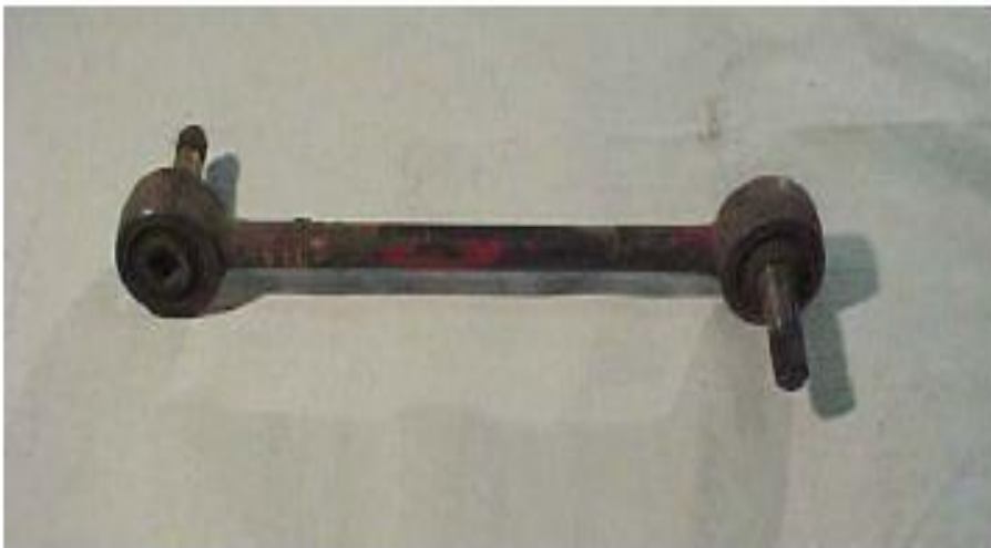
Figure 1. The torque rod assemblies for 2-1/2 and 5 ton 6x6's are very similar. Some of the rods are round from eye to eye (as above) and on some, the shaft between the eyes has an "I-beam" cross section.
