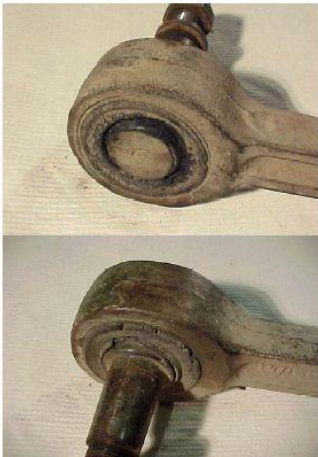
Figure 10. The rubber on the above rod end is beginning to separate from the ball joint. These rod ends should be replaced.
