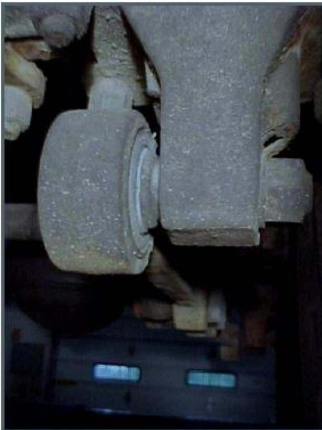
Figure 7. When you inspect the rod ends, always check both the outer and inner sides of them. The rubber of this rod end shows signs of weathering, but no separation from the metal sleeve or ball joint.
