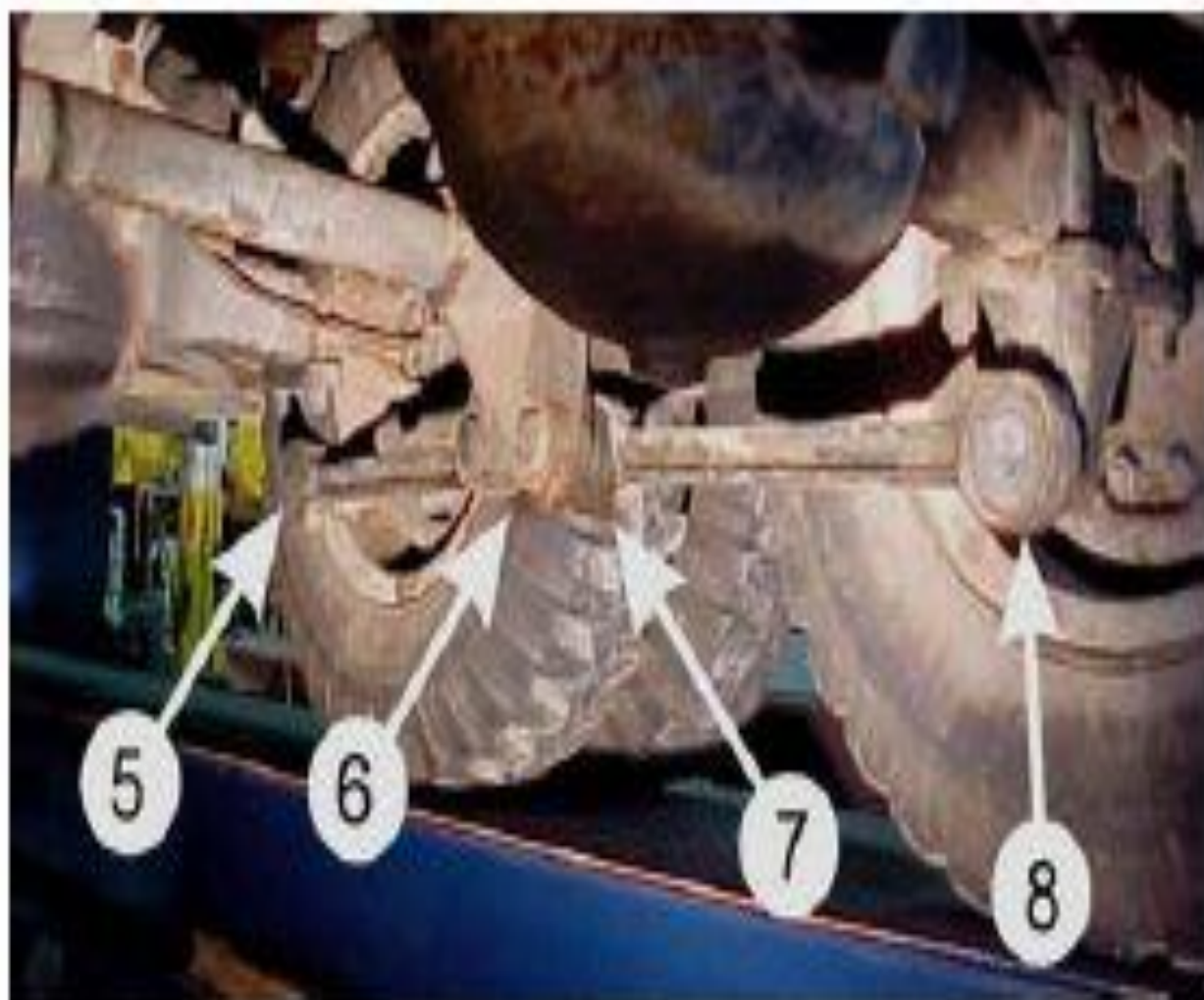
Figure 4. Two lower torque rod assemblies are located on each side of the vehicle. Four rod ends on each side should be inspected.
