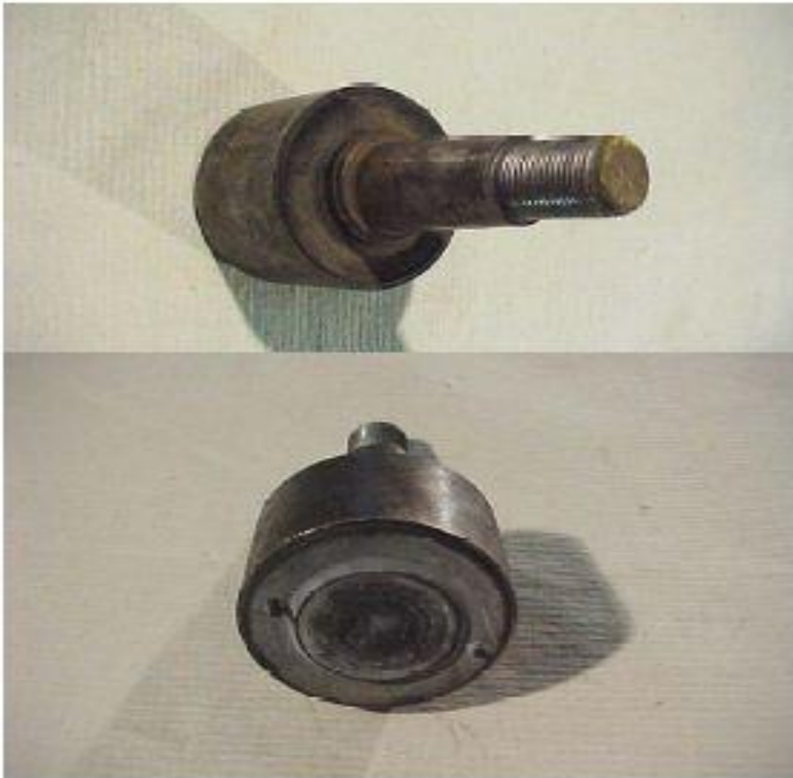
Figure 2. The rod end is a ball joint encased in rubber with a steel outer sleeve. The rod end is pressed into the eye of the rod. The photos above are of a new rod end.
