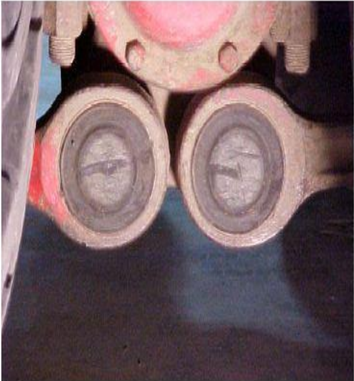
Figure 6. These rod ends have been in service for five to six years. The rubber is still in excellent condition.
