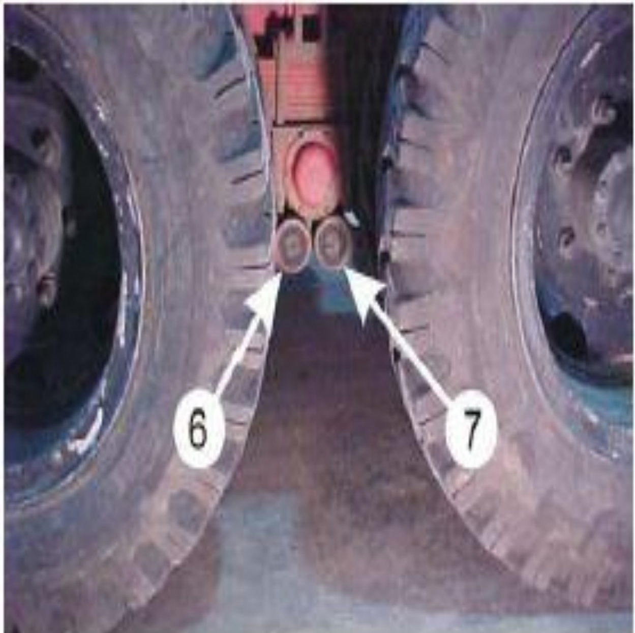
Figure 5. The center two lower rod ends may be easily seen by standing next to the unit and looking between the rear duals.
