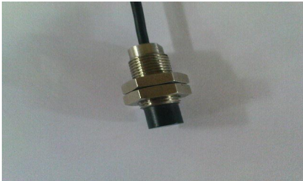
Figure 6.1: Proximity sensor used for experimental modal analysis
