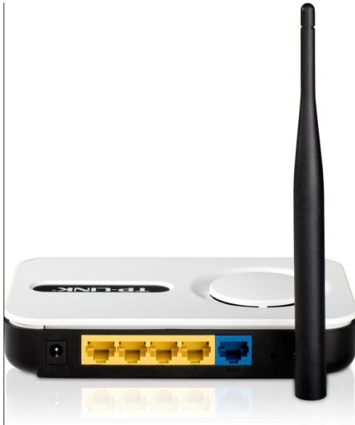
Figure 2.16: TP Link Router, TL-WR340GD
