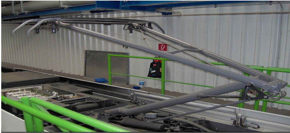
Figure 2.1: (a) The (asymmetrical) 'Z'-shaped pantograph. This pantograph is single-arm.
