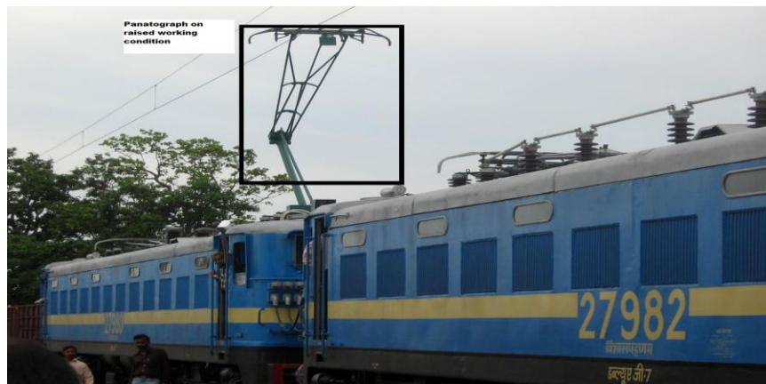
Figure: picture of a pantograph system operating for a high speed train.
