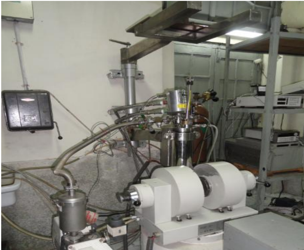
Figure 2.3: VSM setup in the lab
