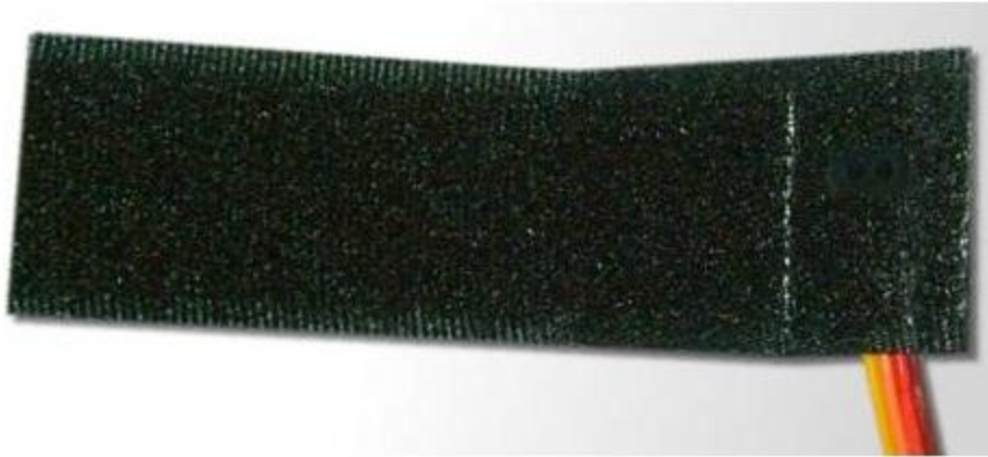
Figure-7.16. IR emitter and detector encased in Velcro
