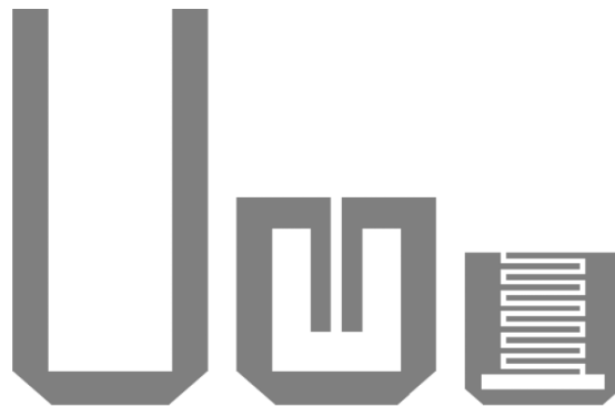
Fig 1.2: (a) Conventional hairpin resonators (b) Miniaturized hairpin resonators using coupled lines (c) Inter digital hairpin resonators.
