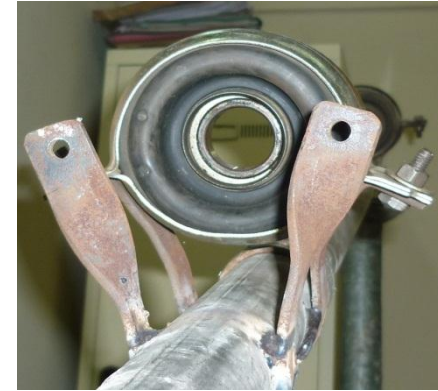
Motor support and bottom bearing
