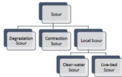
Figure 4: Classification of scour
