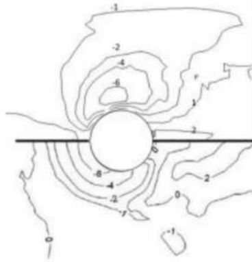
Figure 17: Comparison of experimental (bottom) and numerical (top) bed topography at equilibrium (in cm) for circular shaped pier
