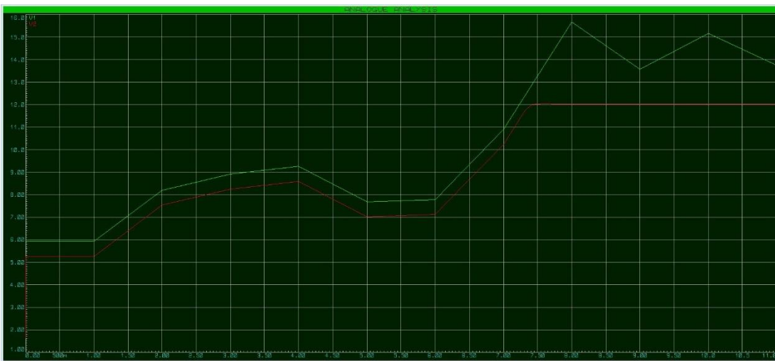
Figure 39. Input and load voltage vs time for two films AEHNB model.
