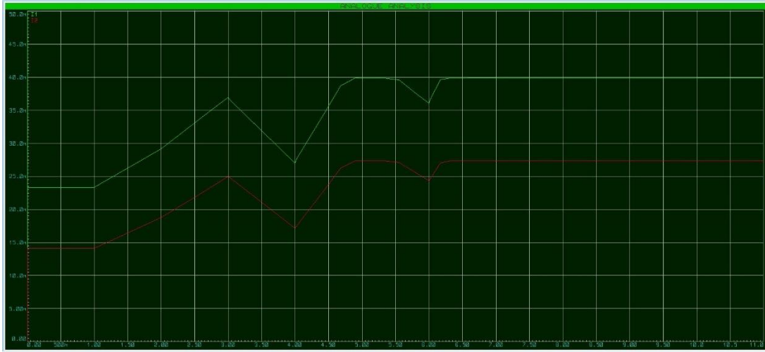
Figure 36. Input and load current vs time plot for one film AEHNB model.
