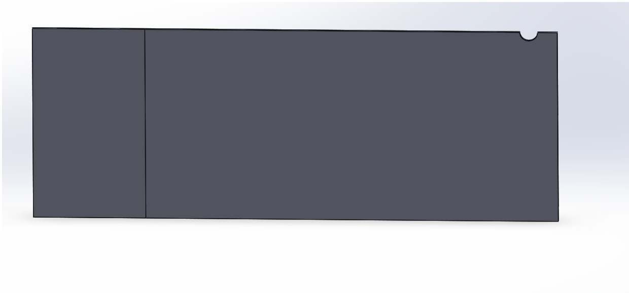
Fig 08: Thin plate with semi-circular crack of volume 28.6 mm 3 where the crack length varies
