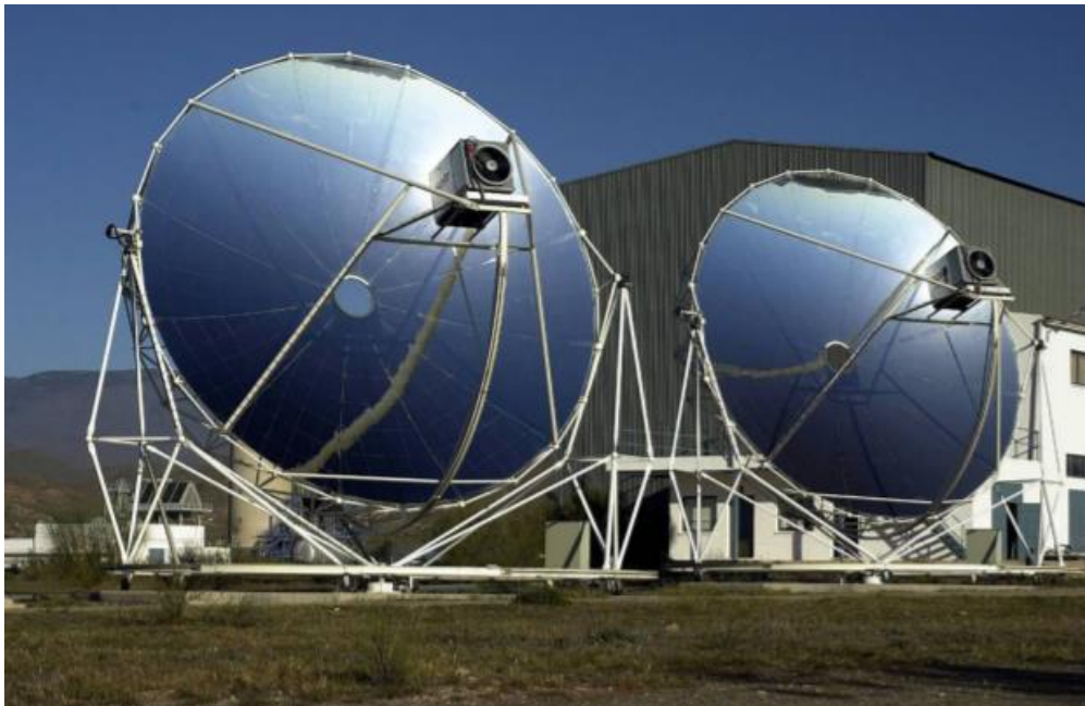
Figure 10: Two units of the 10 kWel EnviroDish installed at the Plataforma Solar de Almeria, Spain. DLR [15]
