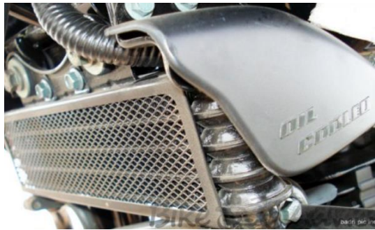
Figure 3.9 A radiator-like system used to cool the oil
