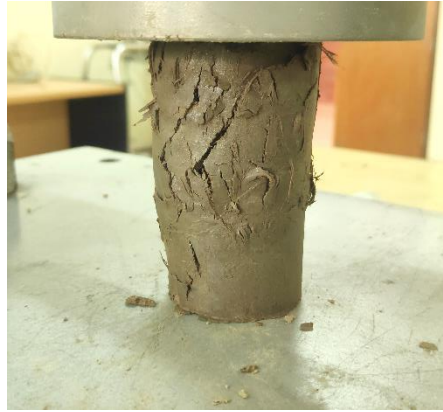
Figure 4.20 Failure Pattern of Soil with 1% betel nut
