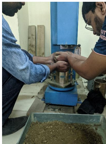
Figure 3.11 Filling up the soil in Compaction Instrument
