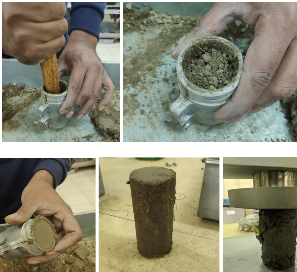
Figure 3.25 UCS Test Procedure of Fiber-reinforced soil
