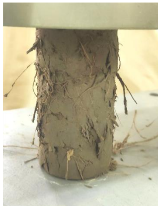
Figure 4.18 Failure Pattern of Soil with 1% Coconut
