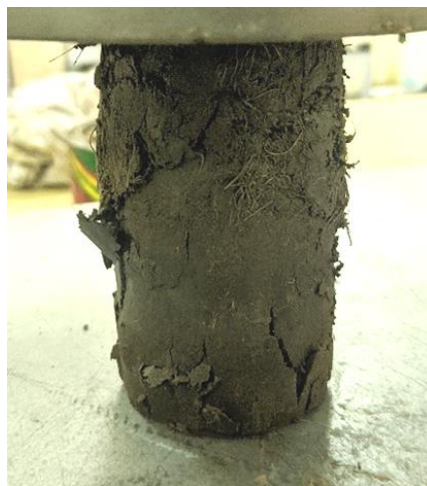
Figure 4.22 Failure Pattern of Soil with 1% Toddy Palm
