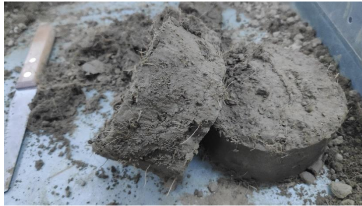
Figure 3.24 Failed Standard Procedure of UCS Test
