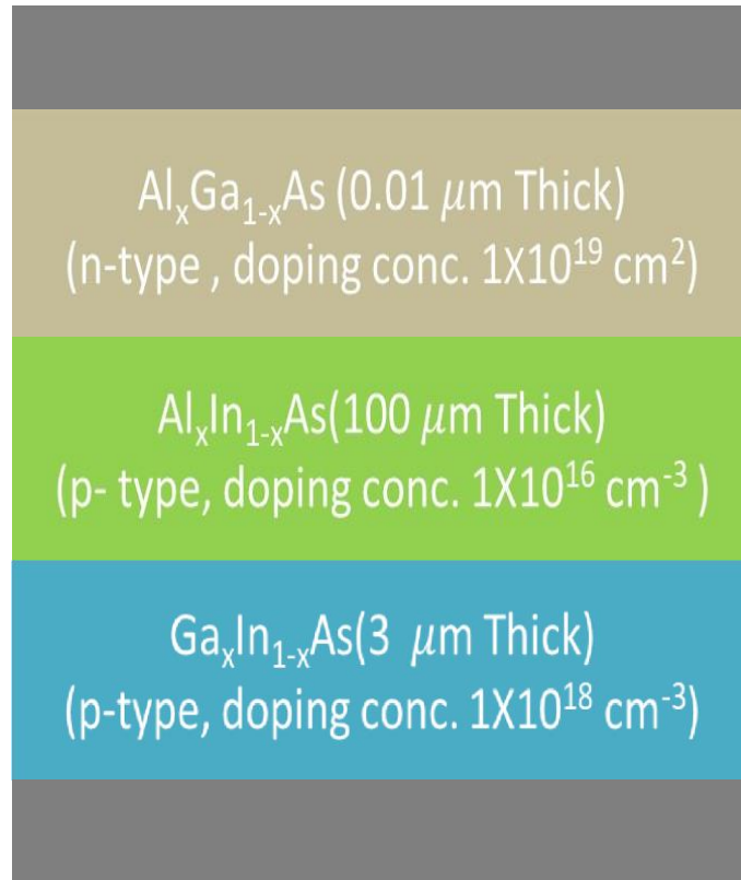
Figure 11: Schematic Diagram of \text{Al}_x\text{Ga}_{1-x}\text{As}/\text{Al}_x\text{In}_{1-x}\text{As}/\text{Ga}_x\text{In}_{1-x}\text{As} Heterojunction solar cell
