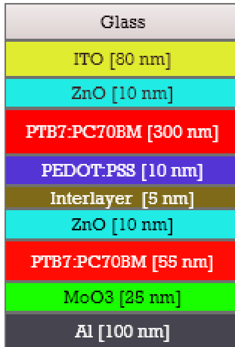
Figure 4-2: Homo structure of PTB7:PC70BM
