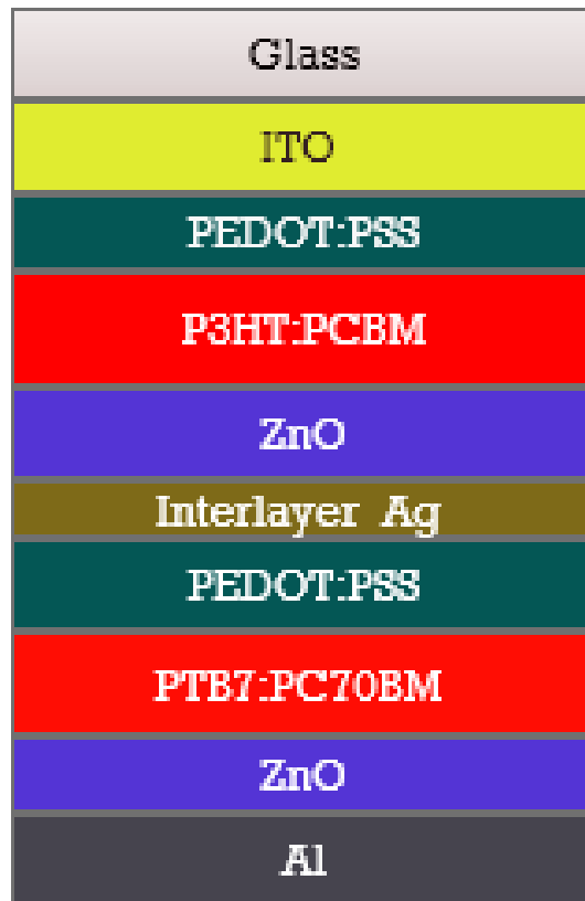
Figure 4-3: Hybrid structure of P3HT:PCBM for top sub-cell and PTB7:PC70BM for bottom sub-cell
