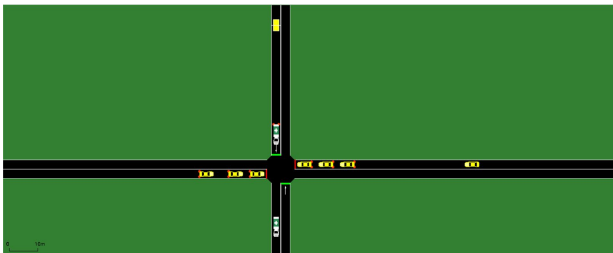
Figure 4 : Emergency vehicles(in white) are given priority whenever they are detected.
