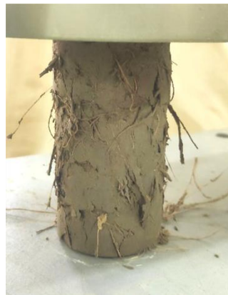
Figure 4.18 Failure Pattern of Soil with 1% Coconut
