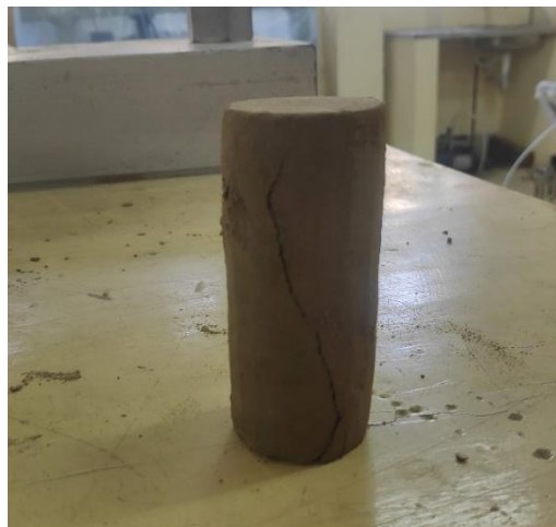
Figure 3.16 Failure Surface after UCS Test
