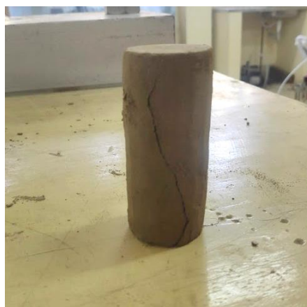
Figure 4.16 Failure Pattern of Soil with no fiber
