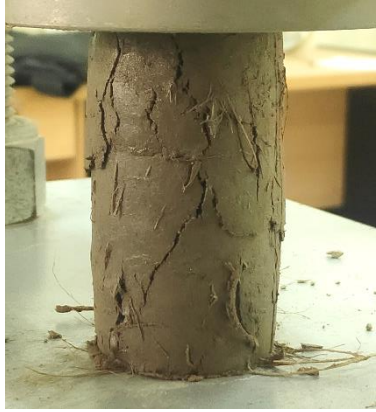
Figure 4.17 Failure Pattern of Soil with 0.5% Coconut
