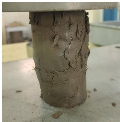
Figure 4.19 Failure Pattern of Soil with 0.5% Betel nut
