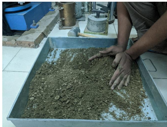
Figure 3.14 Soil Sample preparation with Optimum Water Content
