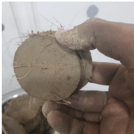
Figure 3.26 Direct Shear test procedure of fiber-reinforced soil
