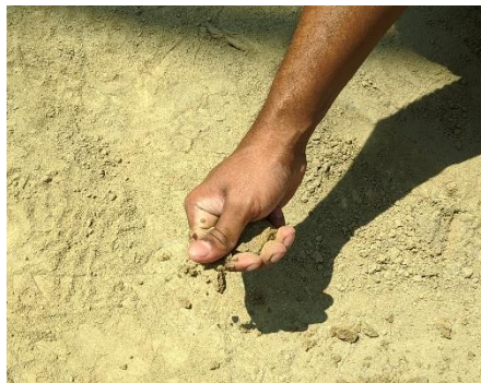
Figure 3.3 Dry Strength Test
