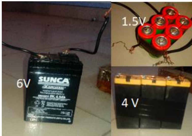
Fig.2.10 Secondary battery bank.
