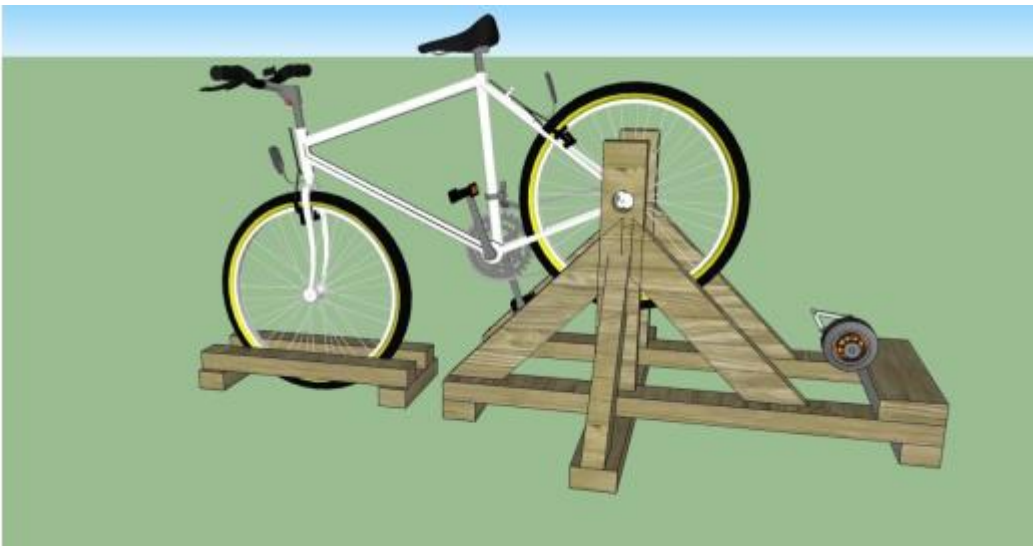
Figure 3.7: Final bike stand design with bike and alternator in place
