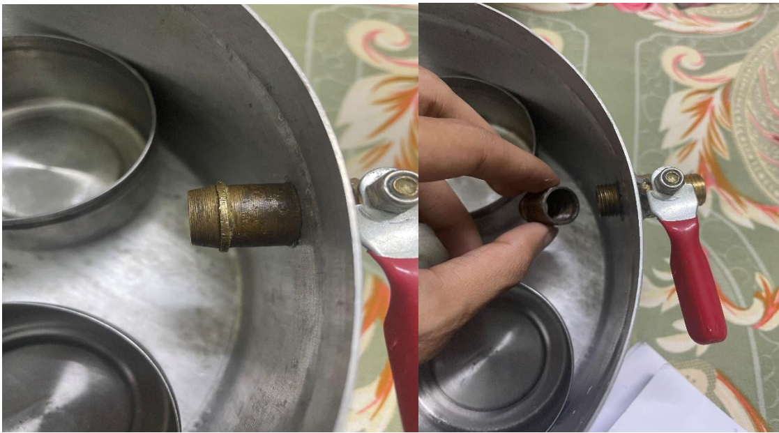
Figure 7: Joint of metal box and valve
