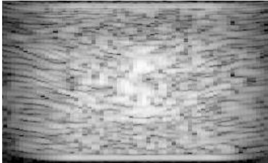
Figure 4.17: Pre-compression B-mode image for the phantom having same background and inclusion properties.
