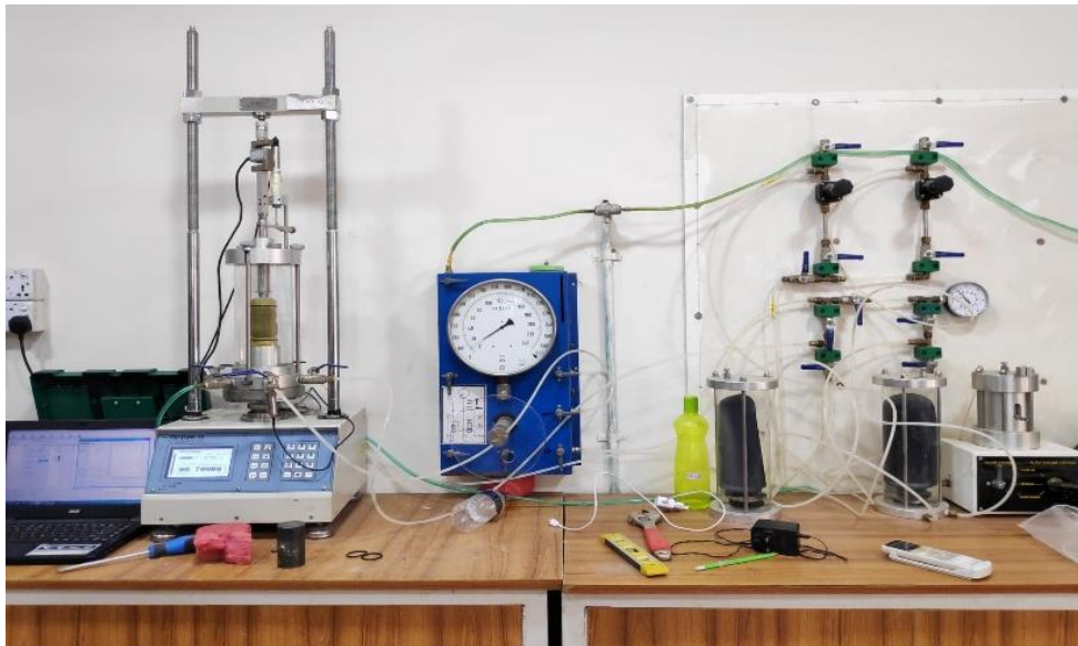
Figure 4.6.1: Tri-axial test at Prosoil Foundation Consultant laboratory
